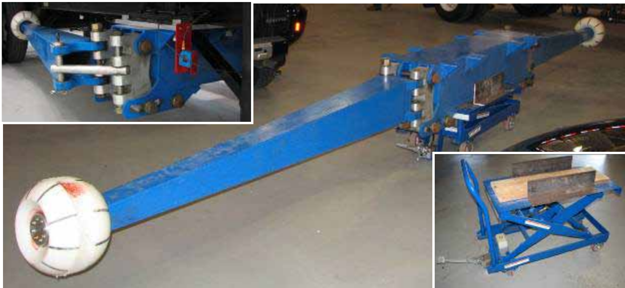
Figure 4.22: Center: completely assembled new NHTSA outriggers ready to go under a trailer. Top Left: picture of the outriggers in transport position. Lower Right: Zorin hydraulic elevating lift cart with payload capacity of 2000lbs and height range of 15.0 - 39.0 inches. It is used to ease the moving and installation of outriggers.
