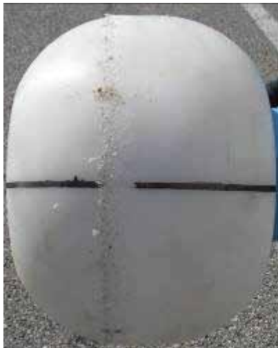
Figure 5.5: Wear after the first observed contact between wheel and test surface.
