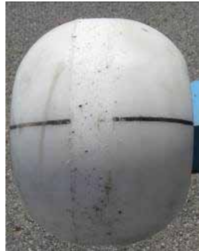
Figure 5.7: Wear after 14 strikes between wheel and test surface. Diameter change is estimated at ~1/32 inch or less.
