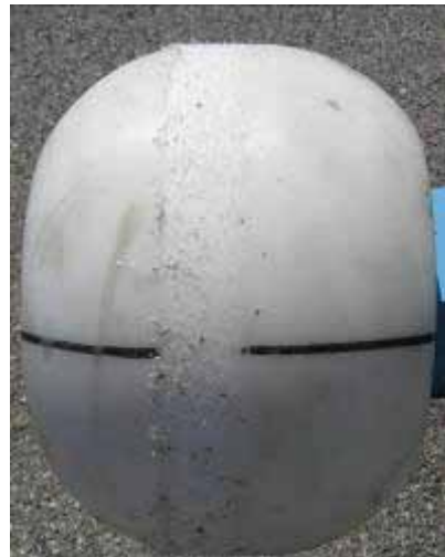
Figure 5.6: Wear after seven strikes between wheel and test surface.
