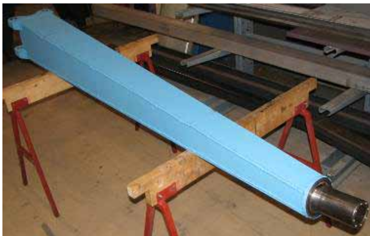
Figure 4.7: Finished welded and painted Outboard Beam.
