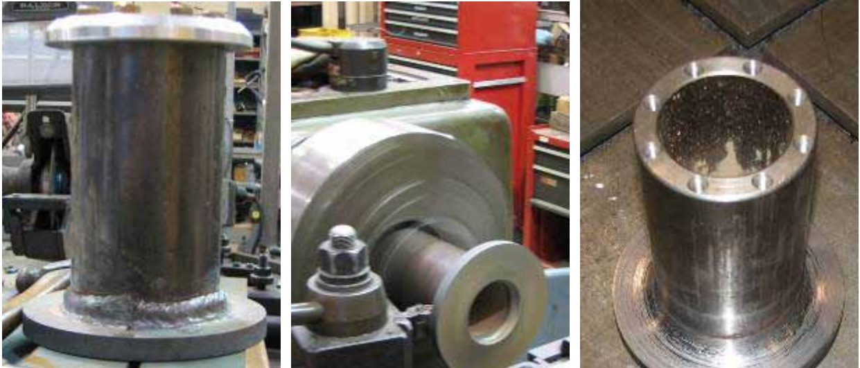
Figure 4.5: Left: End Plate and Axle Shaft are welded together. All inside and outside seams were welded. Middle: the weld bead and face of end plate are turned on a lathe to create chamfer and remove any rough edges that would snag HDPE Plastic Wheel. Right: finished Axle Shaft and End Plate are ready for attachment to Outboard Beam.
