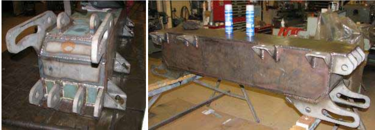
Figure 4.21: Left: 13 th step attachment of Mounting Brackets. Right: final Inboard Beam fabrication; the welds were touched up and cleaned to be painted.
