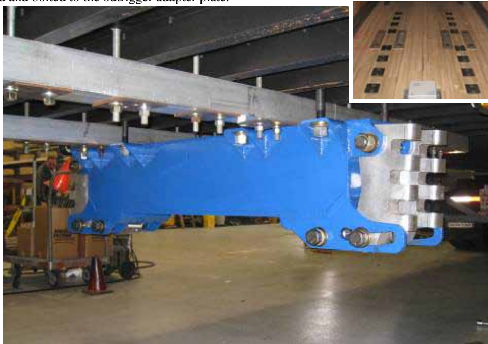
Figure 5.2: Center: Above shows the main beam mounted to a box van type trailer. The aluminum tubes between the outrigger and the bottom of the trailer were added to help distribute forces from the outrigger striking the test surface. Top Right: Inside view of the box van trailer; shows the clamp downs used to hold the aluminum tubes and outrigger to the bottom of the trailer.
