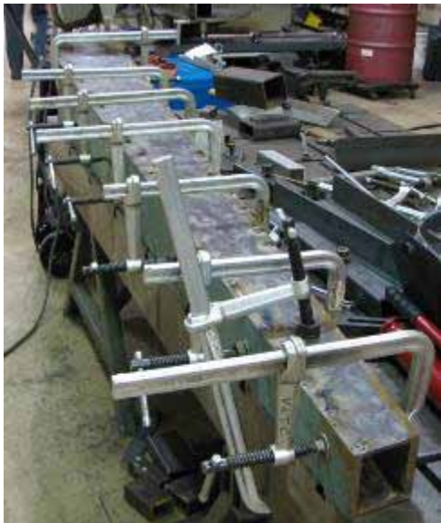
Figure 4.2: Pictures of the fabrication of the outboard beam. Clamps and 90° angle iron pieces are used to jig the plates that form the tapered beam (outer edges are aligned and tacked into place). All outside seams were continuously welded. Inner seams were welded according to what the welder could reach.
