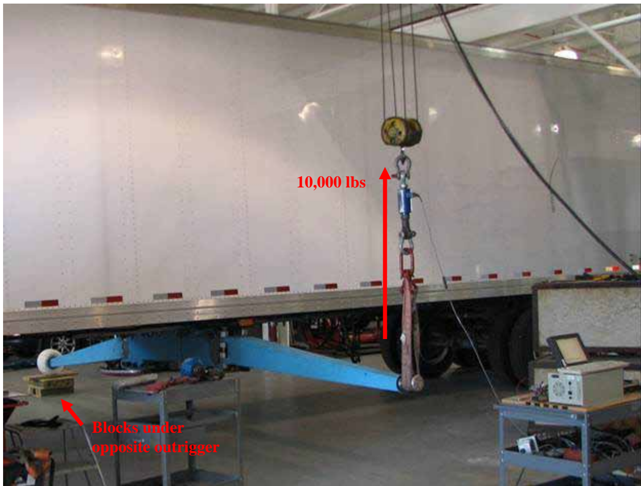
Figure 5.3: Static outrigger and outrigger mount load rating check. Wheel on opposite side is blocked so that both Outboard Beams are evaluated at the same time. The blocks were then removed and a load was reapplied to the outrigger to evaluate the mounts. Setup used an overhead crane and tensile load cell to measure the force applied to the outriggers.
