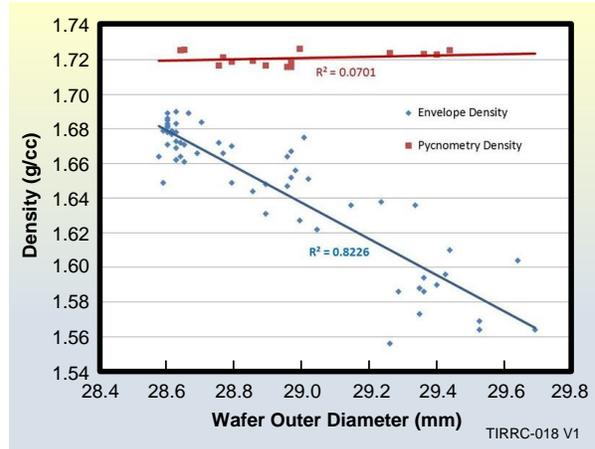
**Figure 17. Density Measurements for 2004 Propellant Wafers.**
