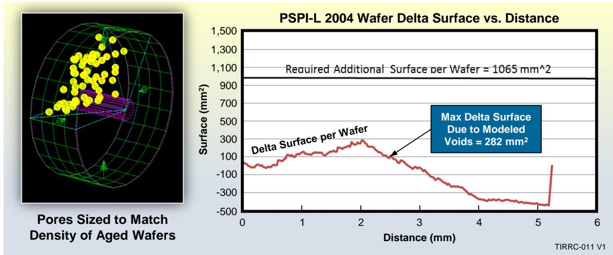
**Figure 10. Closed Pore Impact on Burning Surface.**
