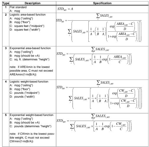
NOTE: Automated curve fitting and optimization only available for function type 2.
