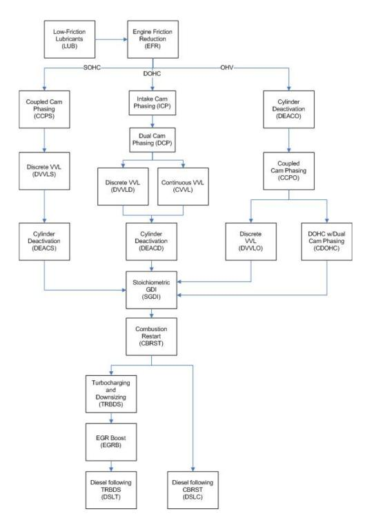
Figure 2. Engine Technology Group Technology Sequence
