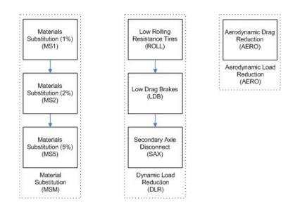
Figure 4. Other Vehicle Technology Sequencing.
