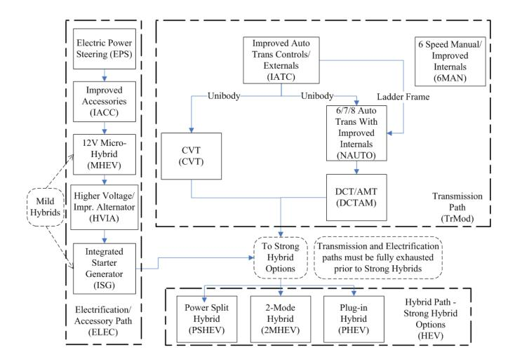
Figure 6. Strong Hybrid Electric Vehicle Options
