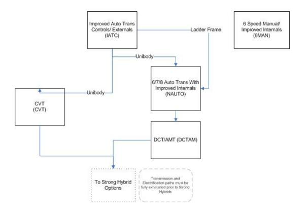
Figure 3. Transmission Technology Group Technology Sequence
