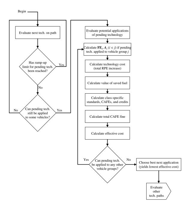
Figure 9. Determination of "Best Next" Technology Application
