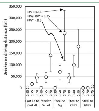
Figure 5. Breakeven driving distance for different material substitution pairs and substitution ratios, assuming different FRV/FRV\* values.
