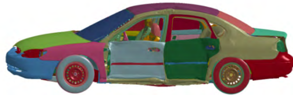
Figure 4-14 – Post-crash deformation of Taurus in side impact
