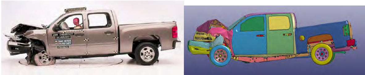
Figure 3-14 – Comparison of post-impact deformation for IIHS ODB test
