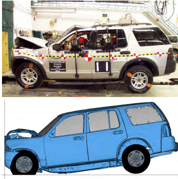
Figure 2-9 – Post-crash images of Explorer after CMVSS 212/301 impact in test and simulation
