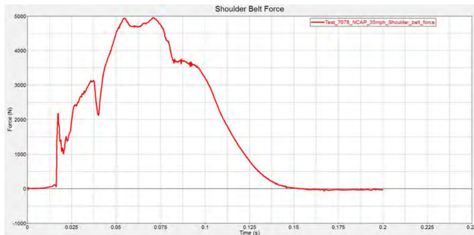
Figure 7-5 – Shoulder belt force for NHTSA test no. 7078
