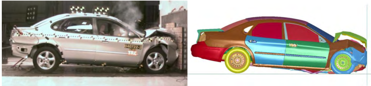
Figure 4-3 – Comparison of the global deformation for Taurus in NCAP test and simulation
