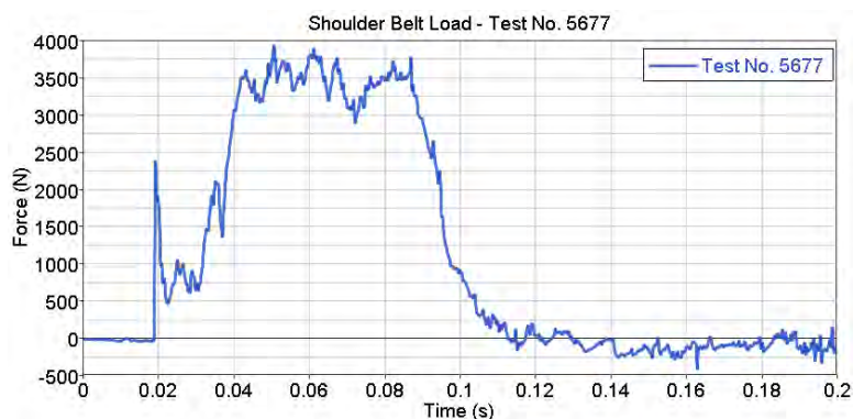
Figure 9-2 – Shoulder belt force for NHTSA test no. 5677
