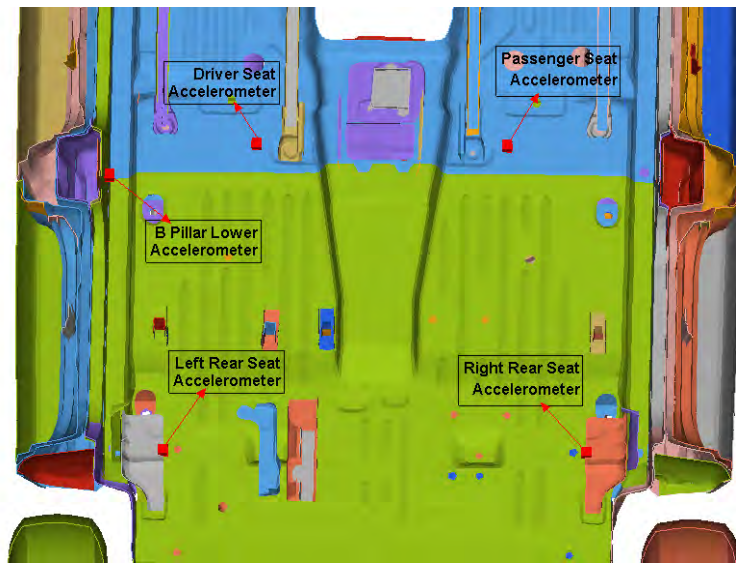
Figure 2-2 – Accelerometer locations in FE model
