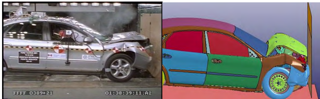
Figure 4-8 – Comparison of the global deformation for Taurus in 30 mph frontal test and simulation
