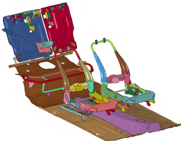
Figure 5-4 – Coarse representations of structural interior components
