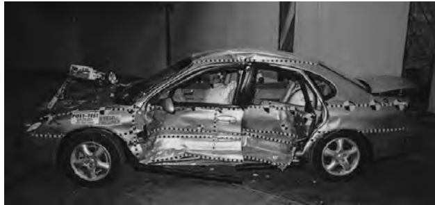
Figure 4-14 – Post-crash deformation of Taurus in side impact
