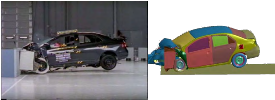
Figure 5-13 – Comparison of post-impact deformation of IIHS ODB test
