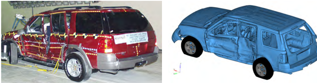
Figure 2-13 – Comparison of post-crash deformation between the side NCAP test and simulation
