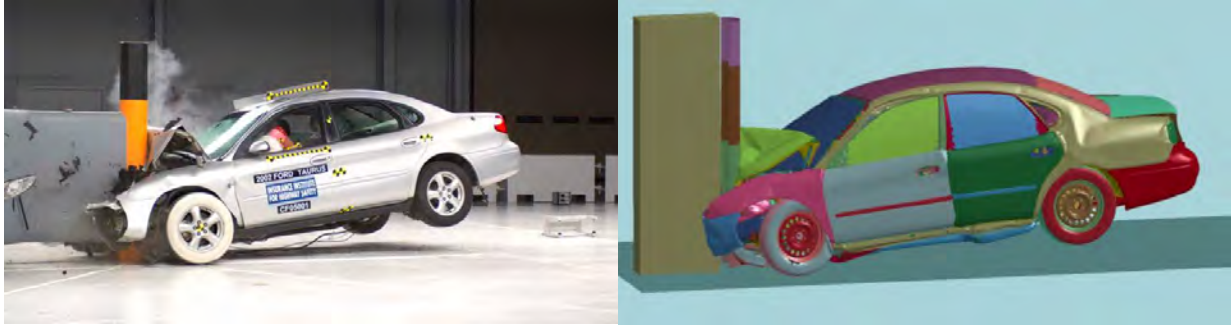
Figure 4-18 – Post-crash images of the Taurus in an offset rigid pole impact
