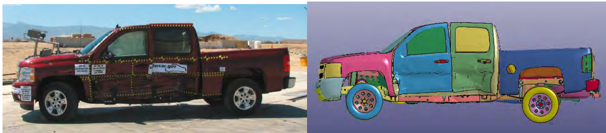
Figure 3-11 – Comparison of deformation post-impact for NCAP side impact test
