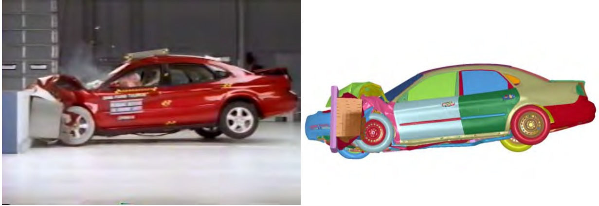
Figure 4-10 – Comparison of post-impact deformation of IIHS ODB test
