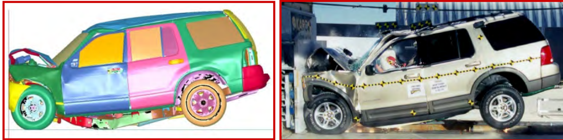
Figure 1-1 – Ford Explorer FEM Structure and Comparison Test
