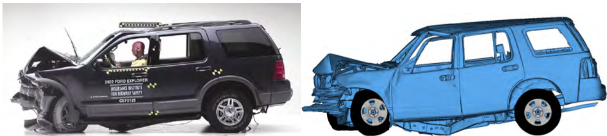
Figure 2-15 – Comparison of post-impact deformation for IIHS ODB test
