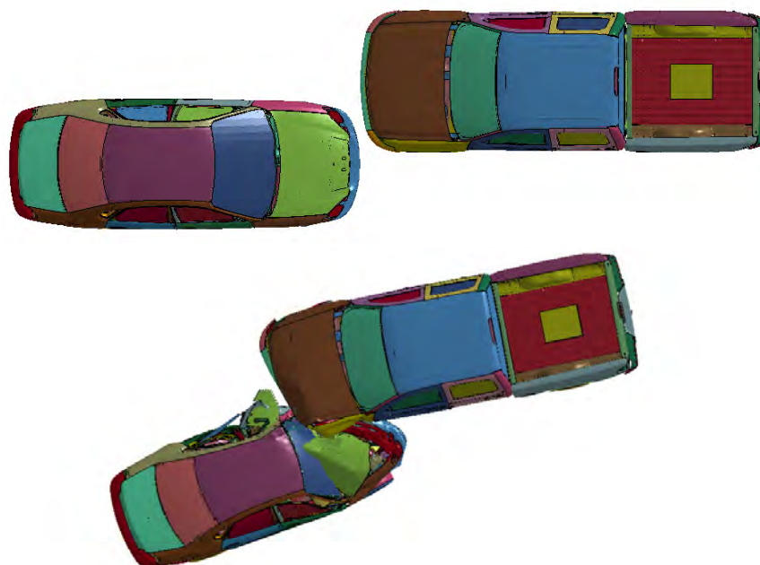
Figure 4-26 – Pre- and post-crash images of the Taurus striking the Silverado with 40 percent overlap
