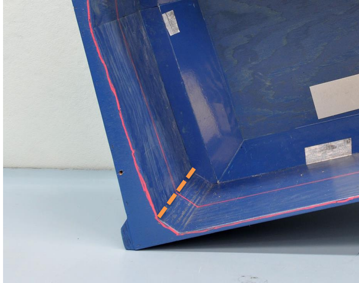
Figure 38. The bottom of the RF_{CRS} structure must fall below the dashed orange line.
