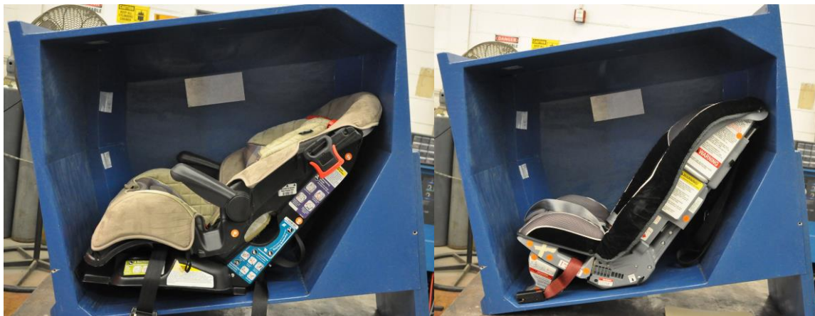
Figure 41. Same RF CRS did not meet bottom contact (left) or angle criteria (right).
