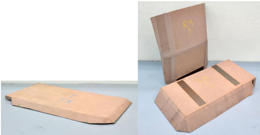
Figure 6. Component added to top of base to make RS_{veh} (left); components added to front and top of RS_{veh} to make RM_{veh} (right).
