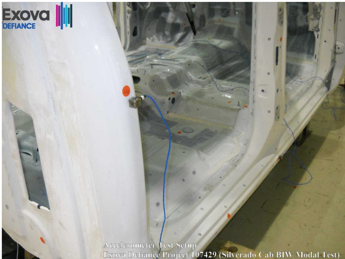
Accelerometer Test Setup Exova Defiance Project 107429 (Silverado Cab BIW Modal Test)
