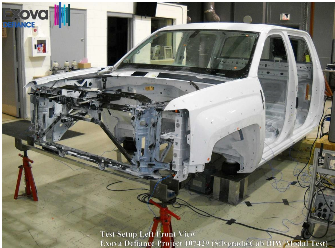
Test Setup Overview Exova Defiance Project 107429 (Silverado Cab BIW Modal Test)
