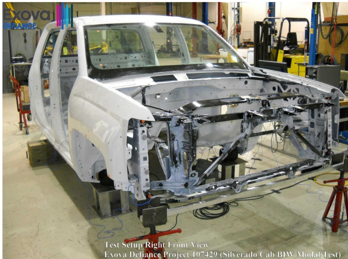
Test Setup Front View Exova Defiance Project 107429 (Silverado Cab BIW Modal Test)
