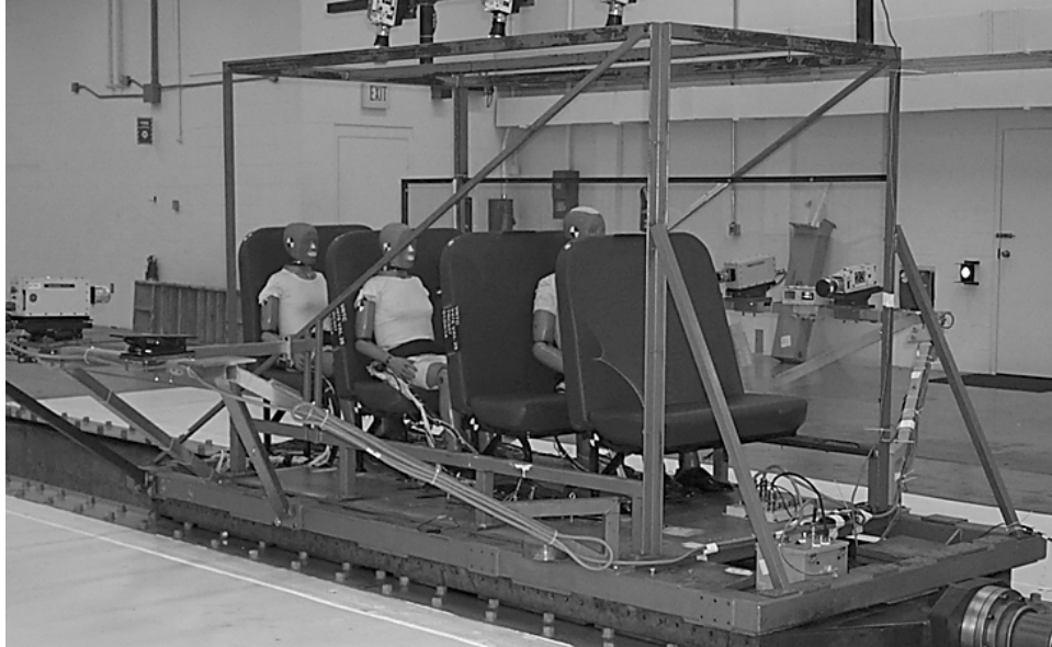
Figure 12. Second Sled Buck used in Frontal Crashes
