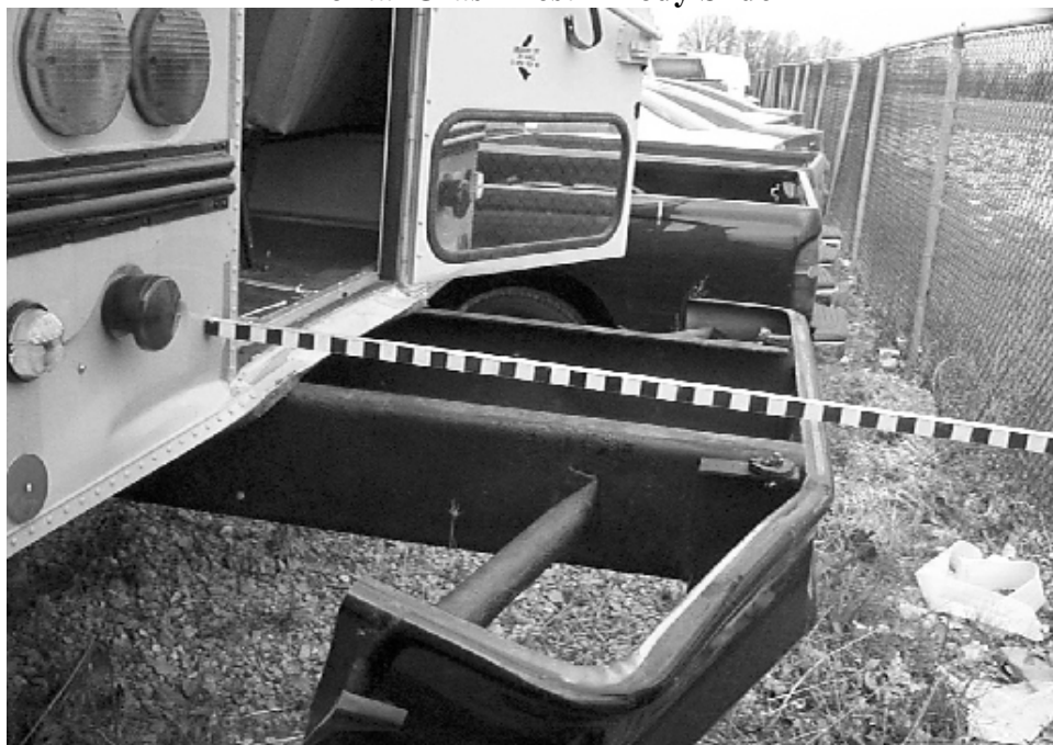
Figure 3. Post-Test Photograph of Frontal Test Showing Body to Frame Movement
