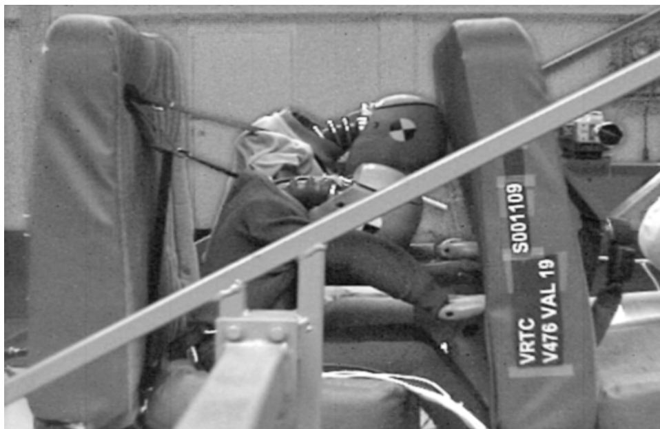
Figure 21. Lap/Shoulder Belt Test at Maximum Neck Flexion
