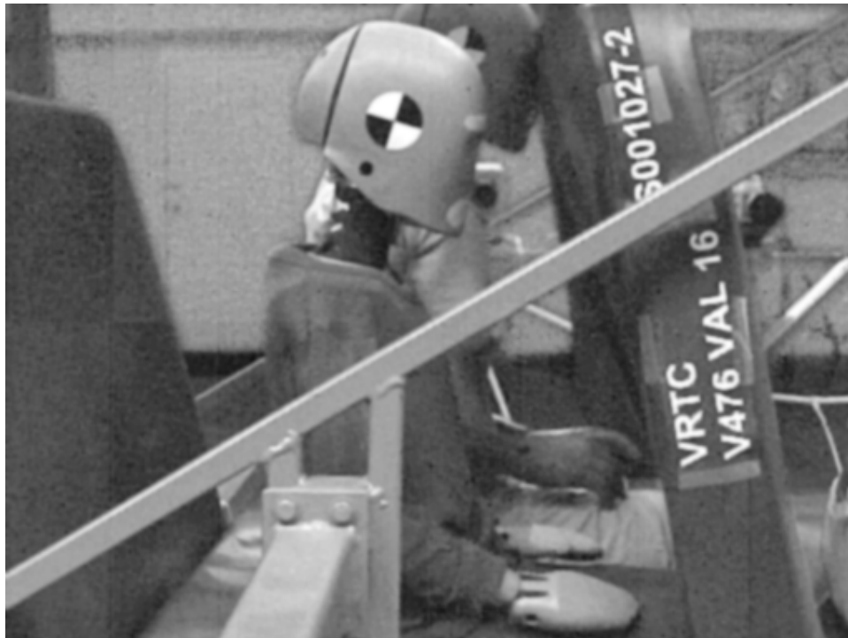
Figure 17. Compartmentalization Test, Knees make Contact with Seat Back at 100 msec
