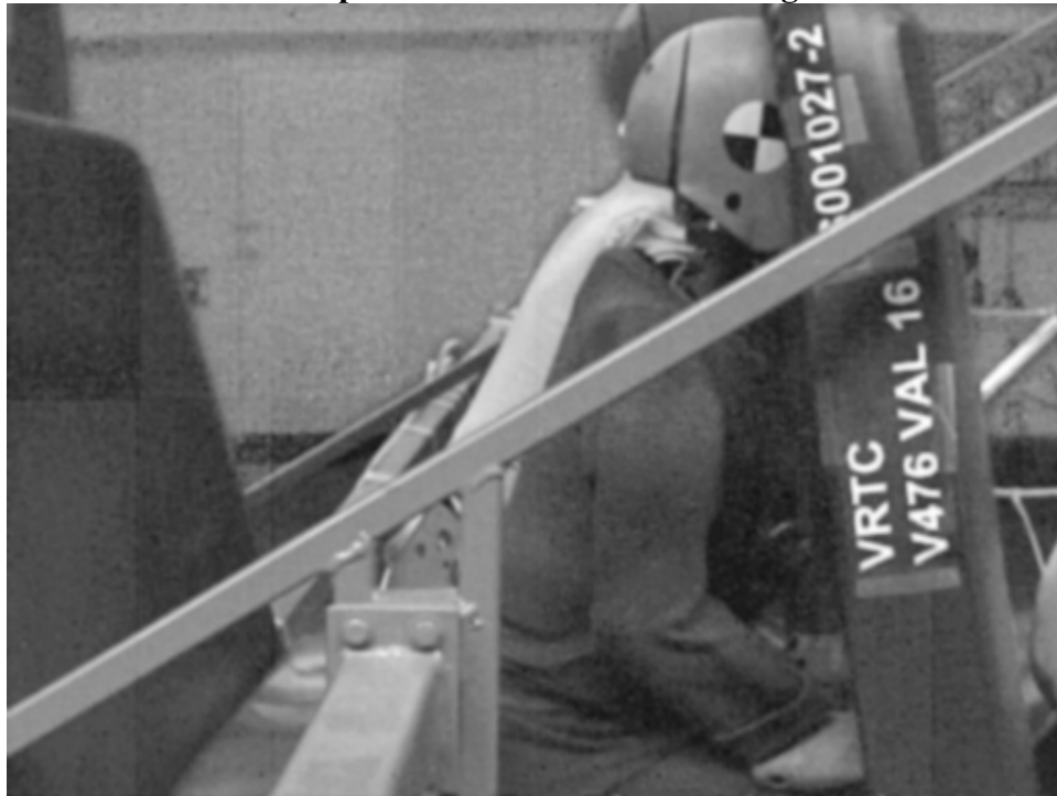
Figure 18. Compartmentalization Test, Upper Body Pivots and Head Contacts at 150 msec
