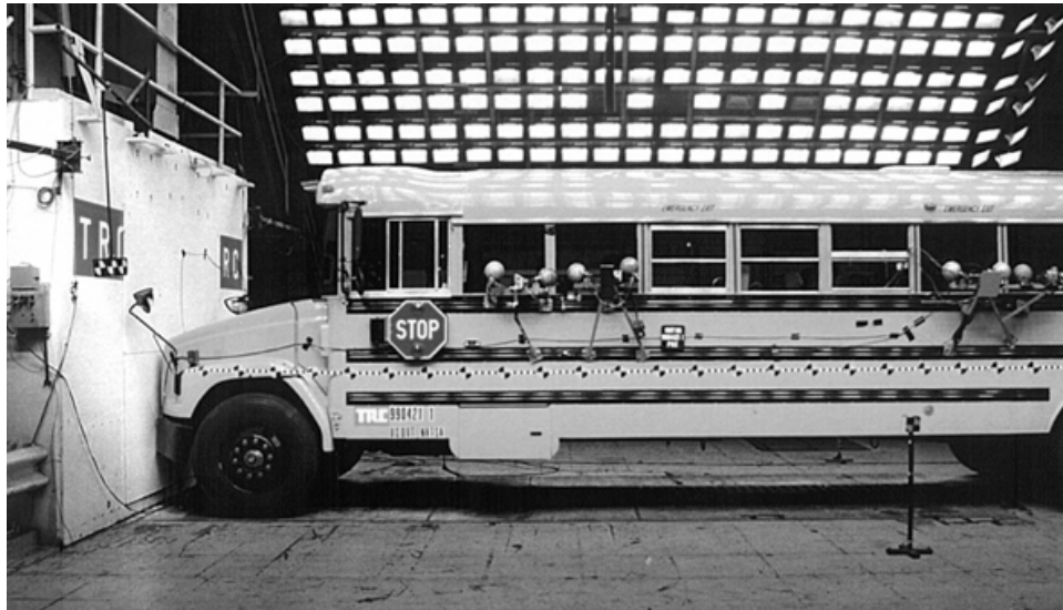
Figure 1. Pre-Crash Photograph of Frontal School Bus Test.
