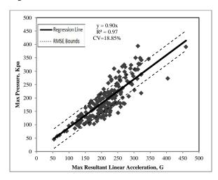
Figure I.2. Max Pressure versus Max Resultant Linear Acceleration.
