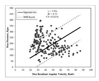
Figure I.4. Max Pressure versus Max Resultant Angular Velocity.
