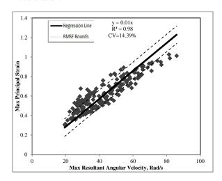
Figure I.12. MPS versus Max Resultant Angular Velocity.
