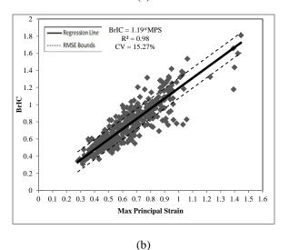
Figure 14. Correlation between (a) BrIC and CSDM and (b) BrIC and MPS for all dummies in available tests (413 data points) using formulation given in equation 4.
