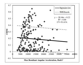
Figure I.7. CSDM versus Max Resultant Angular Acceleration.
