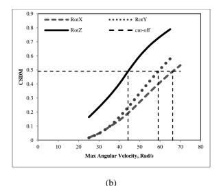
Figure 13. a) Risk of AIS 4+ anatomic brain injury versus CSDM from SIMon model with the cut-off at 50% risk corresponding to CSDM value of 0.49; b) CSDM versus max angular velocity relationships demonstrating that the same risk (at CSDM = 0.49) is achieved at different max angular velocities in different directions.
