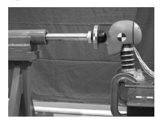
Figure 4. Pendulum test setup. The head and neck assembly of the HIII 50<sup>th</sup> percentile male ATD is shown for a frontal (0 degrees), unpadded impact at the head center of gravity.
