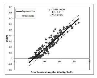
Figure I.8. CSDM versus Max Resultant Angular Velocity.
