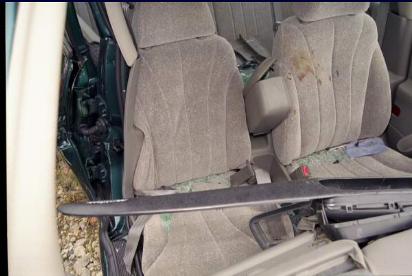
Vehicle 1 – Right front intrusions
