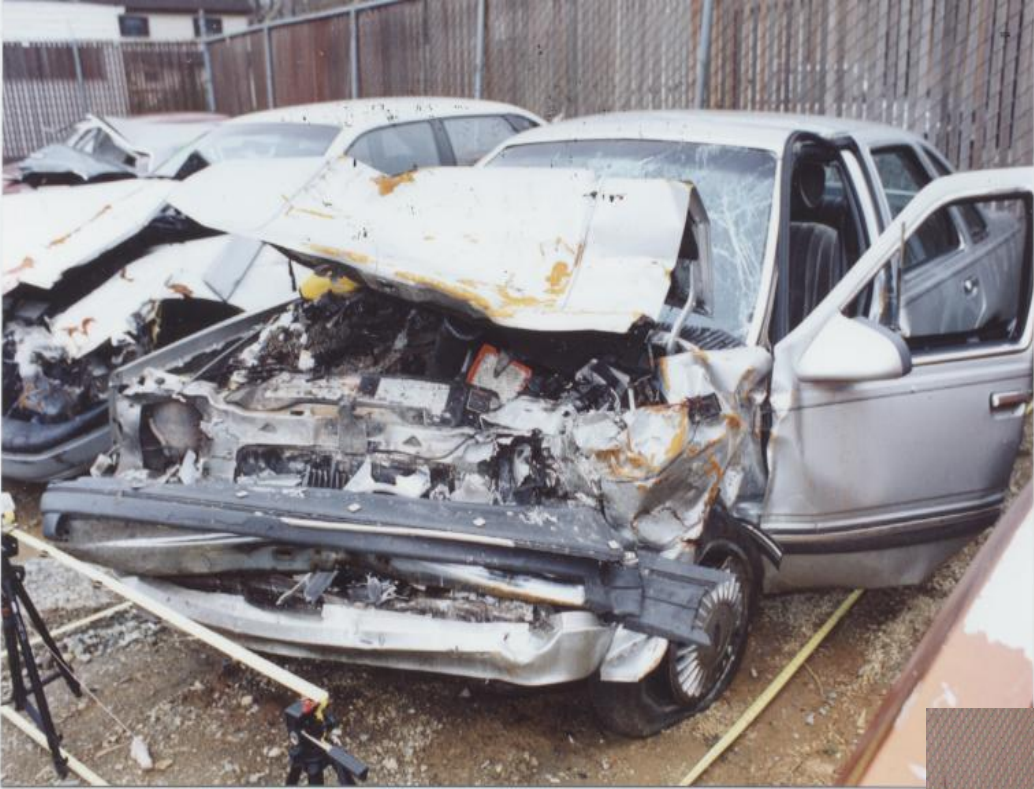
1987 Ford Tempo 1987 Ford Tempo vs. 1980 Oldsmobile Cutlass Total Delta V 35 mph (56 km/h) Weight: 1140 kg
