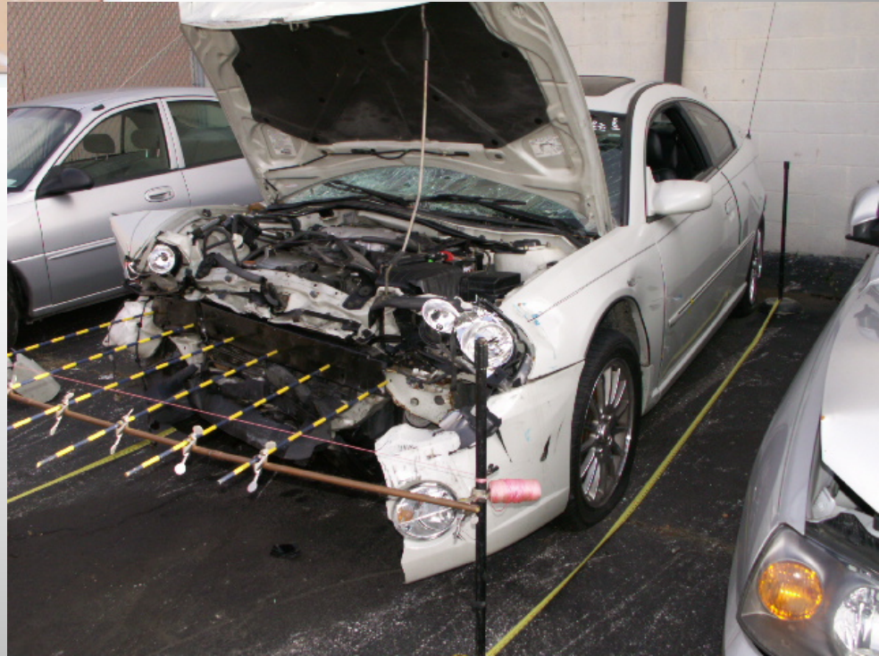
2003 Chrysler Sebring 2003 Chrysler Sebring (2-door sedan) Vs 1997 Chevrolet Cavalier Total Delta V of 38.5 mph (62 km/h) Weight: 1413 kg
