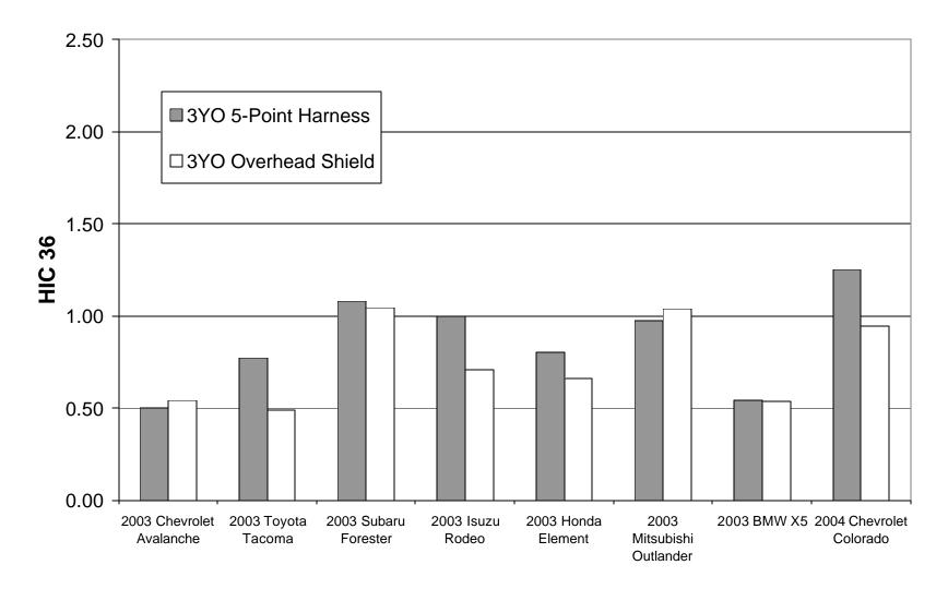
**Figure 7: Normalized HIC Values for Paired Tests**
