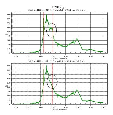
Figure B1: 2003 Mercedes E320 6YO HIC readings, with and without face-to-chest contact
