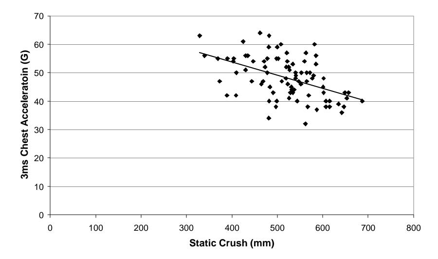
Figure 16: Chest G vs. Static Crush Measurement
