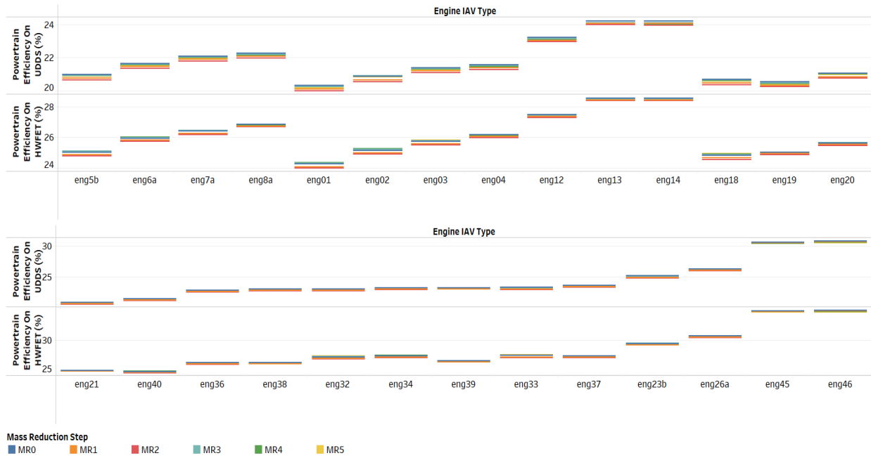
Figure 257. Powertrain efficiency values of different engine types with CVT
