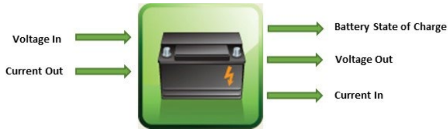
Figure 62. Autonomie energy storage model I/O
