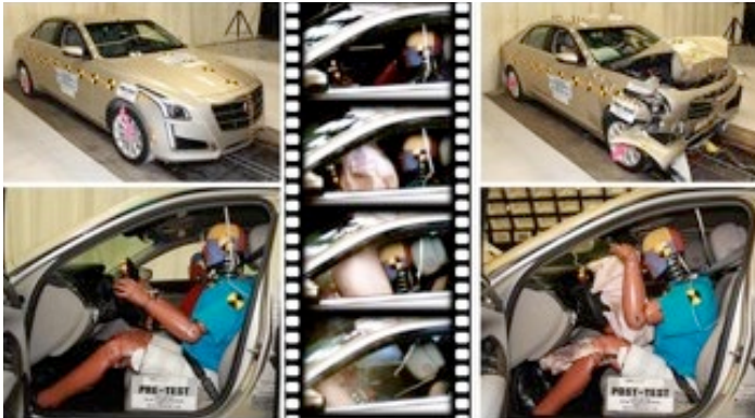
Figure 1. Crash test before, during, and after. Measurements from the test dummy are used to predict the risk of injury to each part of the body.
