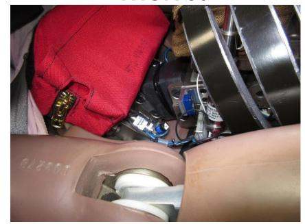
• Side impact ATDs: Changes locations of the head, shoulder and ribs relative to curtains, daylight opening, B-pillar, armrest, door structures
