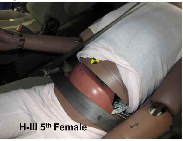
• Large gaps develop between the head and head restraints or shoulder and seat back for certain dummies (with stiffer spine. e.g. H-III)
