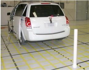
Figure 2. ISO Pole behind Nissan Quest test vehicle.
