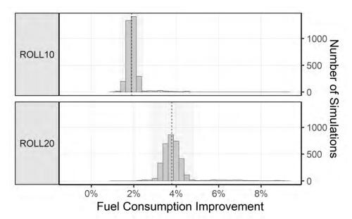
Figure 3-44: HDPUV Roll Technology Effectiveness Values for All Vehicle Technology Classes
