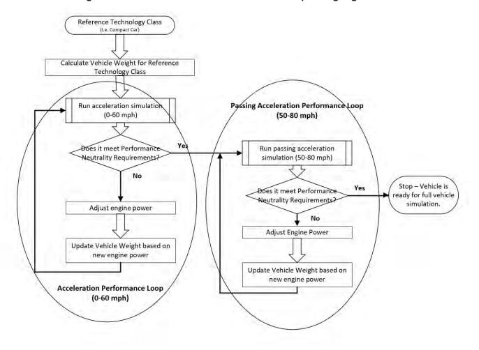
Figure 2-7: Conventional Powertrain Closed Loop Sizing Algorithm
