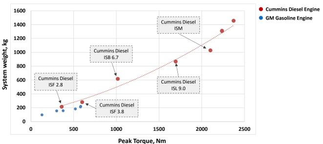
Figure 2-5: HDPUV Engine Mass Determination as a Function of Power and Type of Air Induction and Engine Type
