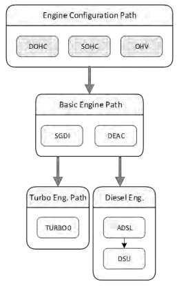
Figure 3-2: HDPUV Engine Technology Paths Available
