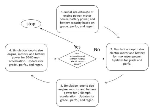
Figure 3-27: Simplified SHEVP2 Sizing Algorithm in Autonomie
