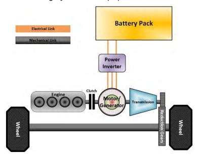
Figure 3-20: Strong Hybrid Parallel (P2) Powertrain Architecture<sup>366</sup>
