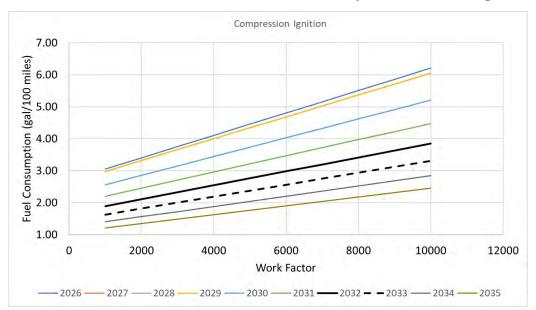
Figure 1-19: Alternative HDPUV14, HDPUV Fuel Efficiency – CI Vehicles, Target Curves
