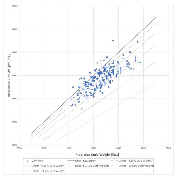
For points with actual curb weight below the predicted curb weight, we use the residual as a percent of predicted weight to get a sense for the level of current MR technology used in the vehicle. Notably, vehicles approaching -20 percent curb weight widely use advanced carbon fiber composites throughout major vehicle subsystems, and few examples exist in the MY 2022 fleet.<sup>595</sup>
