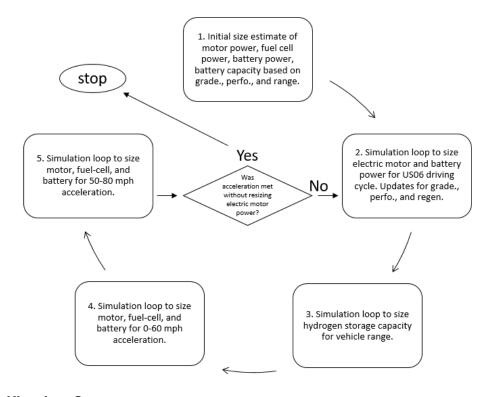
Figure 3-30: Simplified Fuel Cell Vehicle Sizing Algorithm
