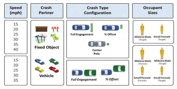
For vehicle-to-vehicle impact simulations, four finite element models were chosen to represent the fleet as shown in Table 7-29. The partner vehicle models were selected to represent a range of vehicle types and weights. It was assumed vehicle models would reflect the crash response for all vehicles of the same type, e.g., mid-size car. Only the safety or injury risk for the driver in the target vehicle and in the partner vehicle were evaluated in this study.
