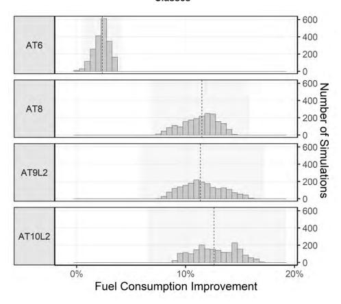
Figure 3-17: HDPUV Transmission Technology Effectiveness Values for All Vehicle Technology Classes
