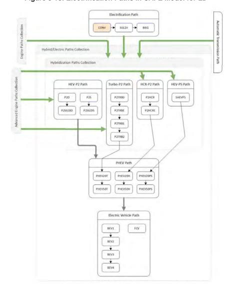
Figure 3-18: Electrification Paths in CAFE Model for LD
