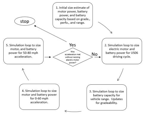
Figure 3-29: Simplified BEV Sizing Algorithm in Autonomie
