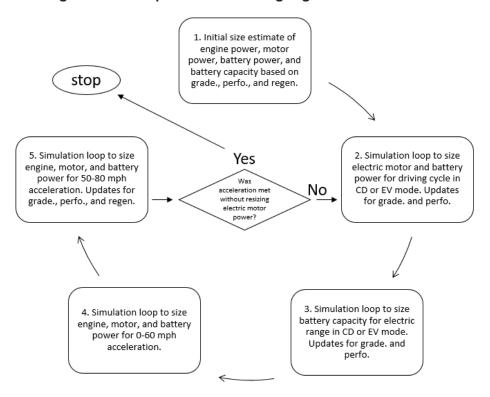
Figure 3-28: Simplified PHEV Sizing Algorithm in Autonomie
