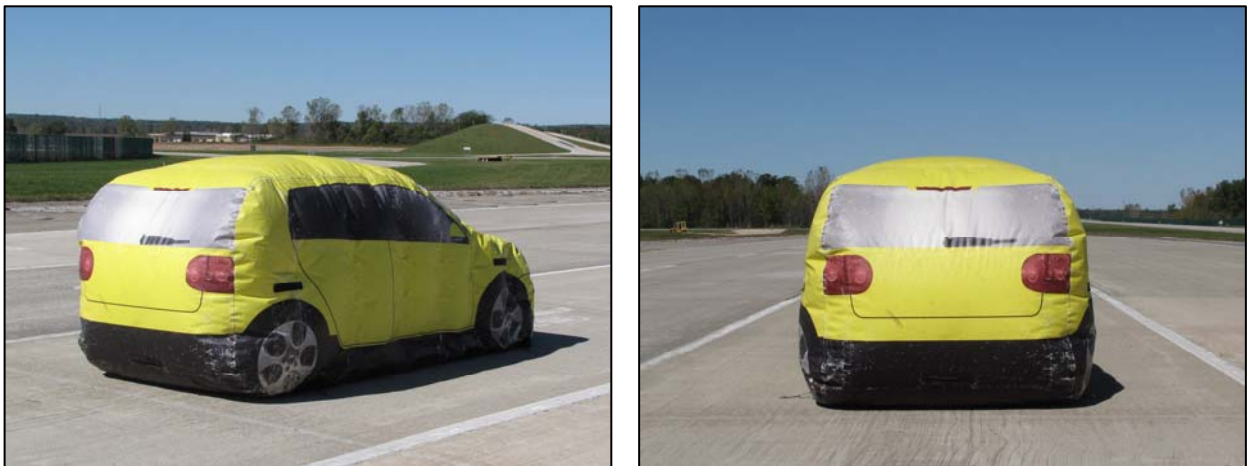
Figure 3.3. Inflatable balloon car, used at the stationary lead vehicle in this study.
