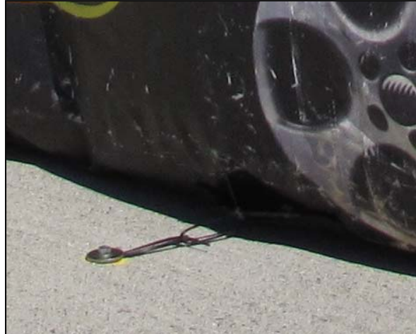
Figure 3.4. Stationary lead vehicle restraint anchor.
