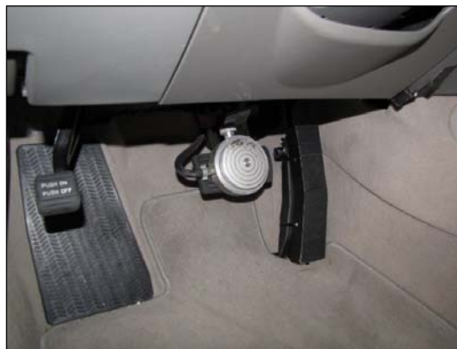
Figure 3.7. Load cell used to measure brake force. Note adapter to increase throttle step height.
