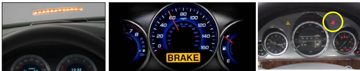
Figure 1.1. Visual alerts presented by the Volvo S80, Acura RL, and Mercedes E350 (from left to right).
