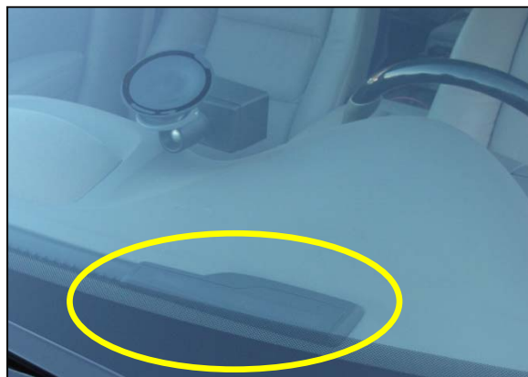
Figure 3.5. Volvo S80 FCW HUD hardware installed in the subject vehicle dashboard.
