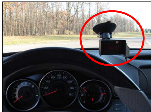
Figure 3.6. Headway monitor installed in the SV.
