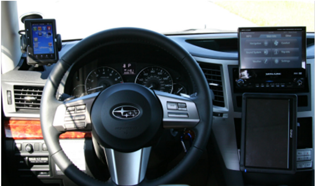
Figure 6-2. Experiment vehicle interior showing OEM display, portable display, and response touchpad
