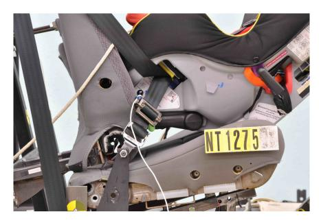
Figure 23. Child restraint installed with gap to achieve same initial angle achieved under FMVSS No. 213 conditions
