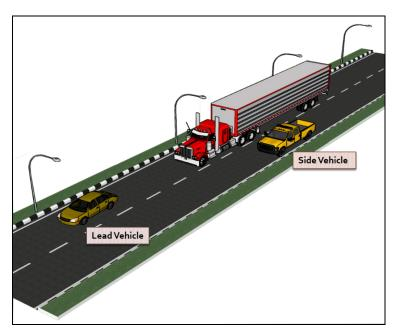
Figure 12. Vehicle Placement during Test Trials
