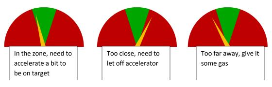
Figure 34. Illustration of Revised Headway Display
