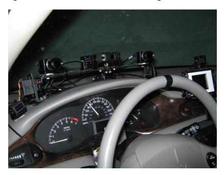
Figure 6. Face Lab Cameras Mounted in the Malibu Cab with a Separate Head Tracking System
