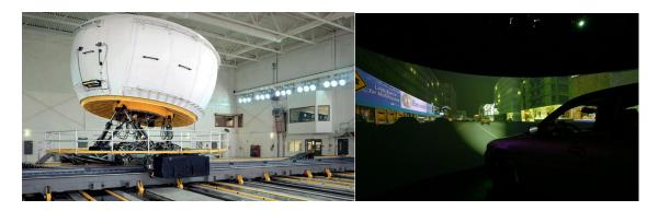
Figure 5. Representation of NADS-1 Driving Simulator (left) with a Driving Scene from Inside the Dome (right).
