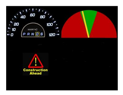
Figure 3. Headway Display Gauge (Upper Right); Early Alert Icon (Lower Left)
