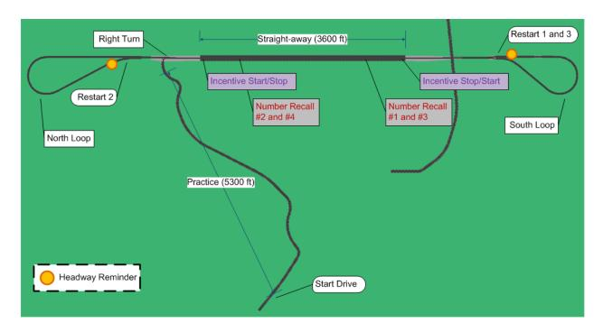
Figure 9. Replica Test Track Road Network
