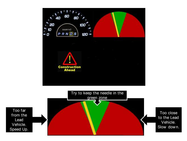
Figure 4. Headway Display Gauge (Upper Right)
