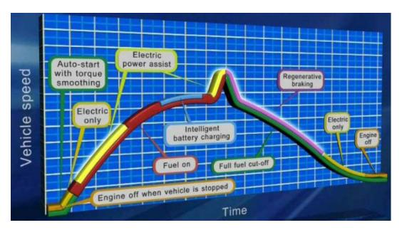
Figure 23 - Hybrid Electric Vehicle Principles [source: www.gm.com]
