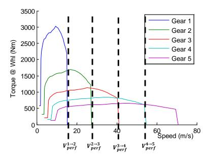
Figure 28 - Maximum Engine Torque at Wheels and Performance Upshift Speeds
