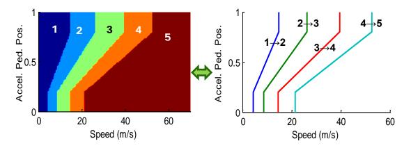
Figure 26 - Upshifting Gear Map (left), Upshifting Vehicle Speeds (right)
