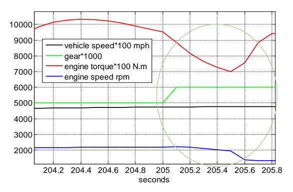
Figure 31 – Torque Hole in Autonomie during Shifting Event
