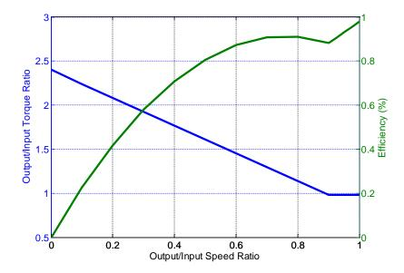
Figure 35 - Torque Converter efficiency
