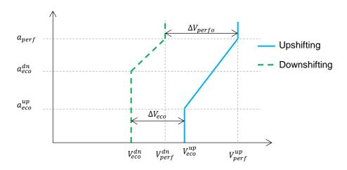
Figure 29 - Design of Upshifting and Downshifting Speed Curves for Two Adjacent Gears
