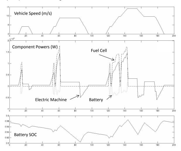
Figure 43 – Component Operating Conditions of a Fuel Cell Vehicle on the Urban European Drive
