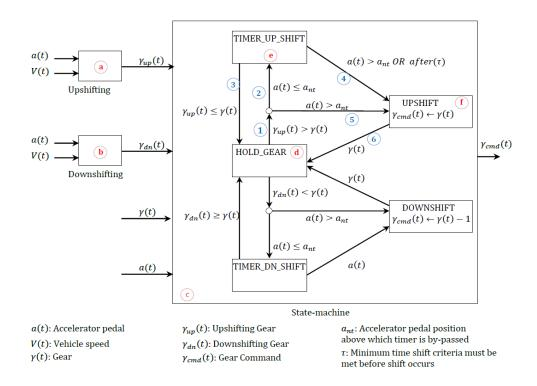
Figure 25 - Shifting Controller Schematic
