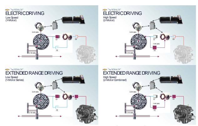
Figure 42 - Voltec Operating Modes [www.gm.com]
