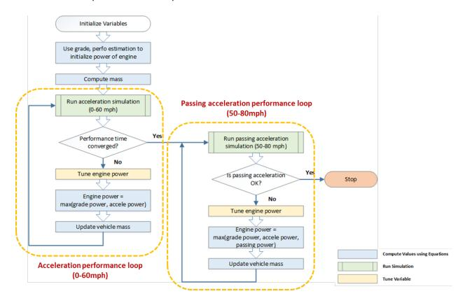
Figure 57 - Conventional Powertrain Sizing Algorithm
