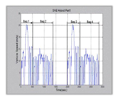
Figure 46 - The urban cycle for a hybrid vehicle
