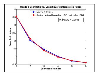
Figure 15 - Comparison of Actual Gear Ratios and Gear Ratios Calculated
