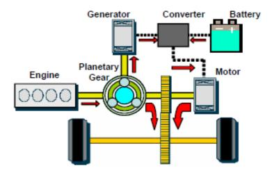
Figure 20 - Power Split Hybrid Electric Vehicle
