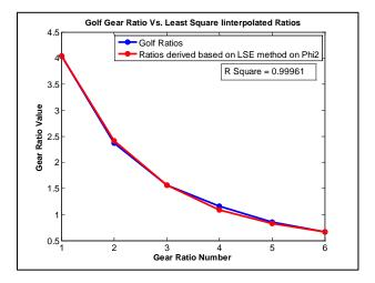
Figure 16 - Comparison of Actual Gear Ratios and Gear Ratios Calculated
