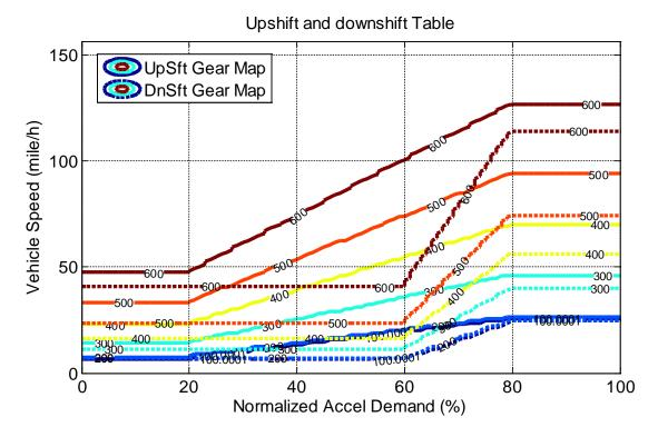
Figure 33 - 6-speed automatic up (plain lines) and down (dotted lines) shifting map
