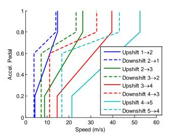
Figure 24 - Shifting Speed Curves for Light-Duty Vehicle in Autonomie
