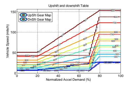
Figure 34 – 8-speed automatic up (plain lines) and down (dotted lines) shifting map
