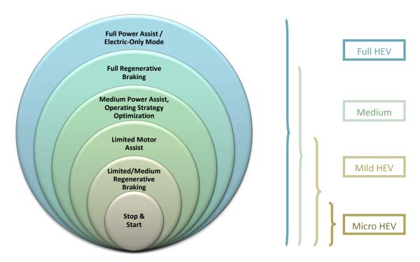
Figure 18 - Electric Drive Configuration Capabilities
