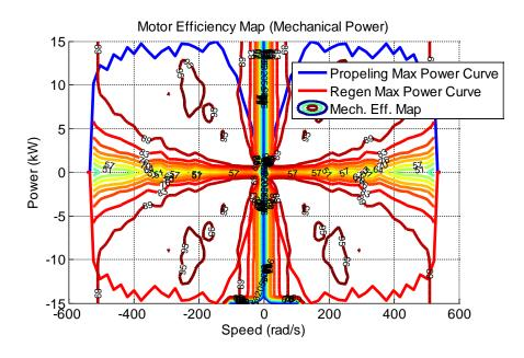
Figure 37 - Electric Machine Map for Micro- and Mild HEV
