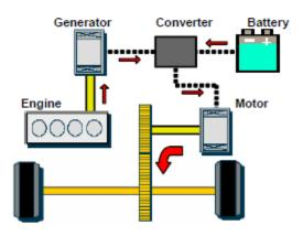
Figure 19 - Series Hybrid Electric Vehicle
