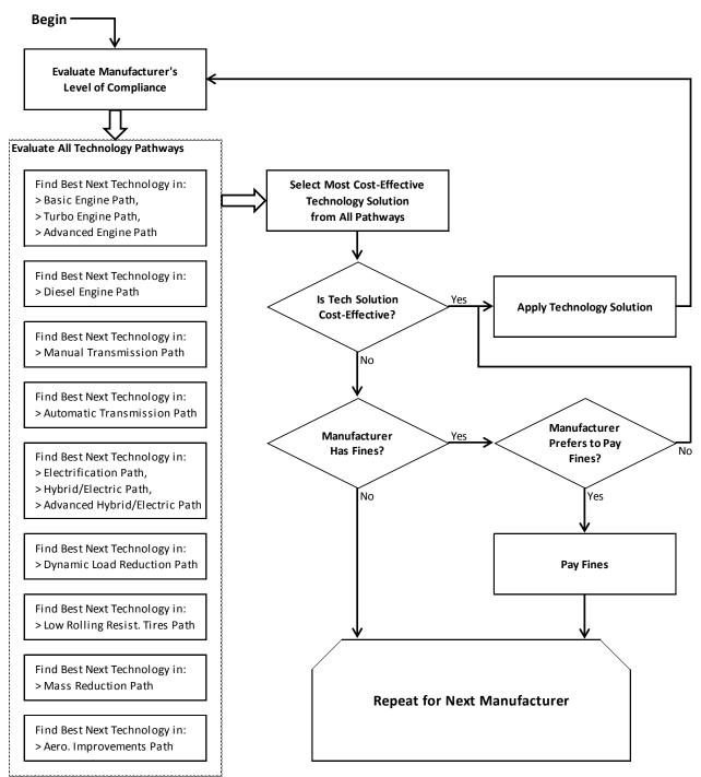
**Figure 7. Compliance Simulation Algorithm**
