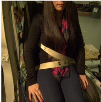
M4-2 Lap buckled shoulder belt under arm.
