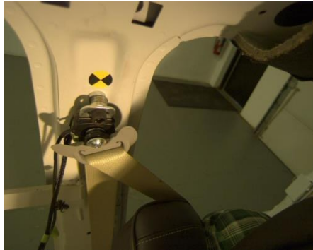
M4-2 Lap buckled, shoulder belt under arm.
