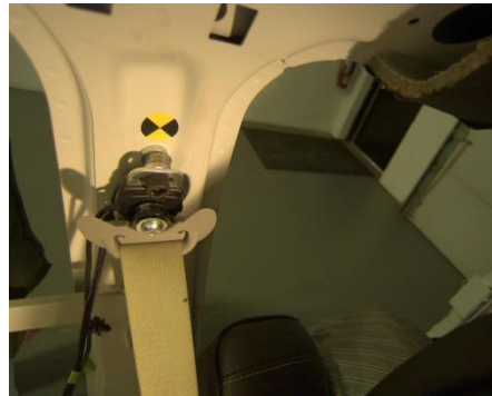
M5-1 Lap buckled, shoulder belt behind seat.
