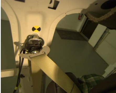
M4-1 Lap buckled, shoulder belt behind back.
