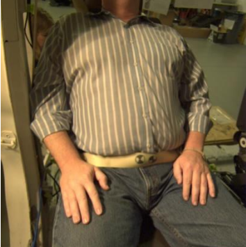
M4-1 Lap buckled, shoulder belt behind back.
