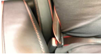
Shoulder belt behind user (lap belt in correct position). Occupant buckled.
