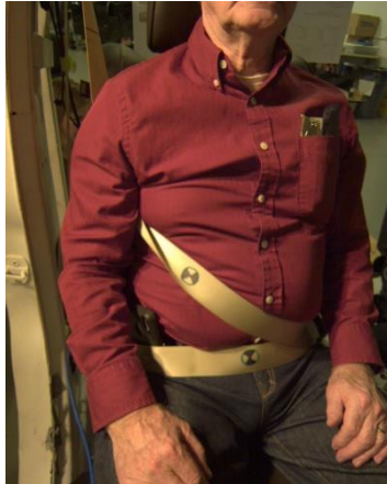
M4-2 Lap buckled, shoulder belt under arm.
