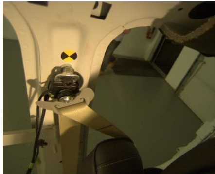
M4-2 Lap buckled, shoulder belt under arm.
