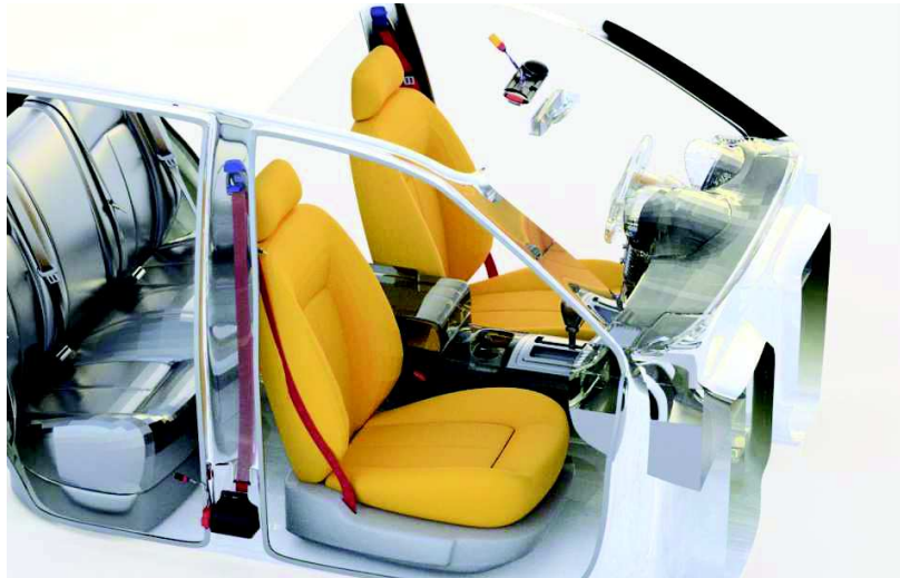
Concept System 9 Vision system with retractor spool payout sensors and with a smart buckle switch
