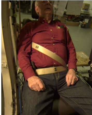
M4-2 Lap buckled, shoulder belt under arm.
