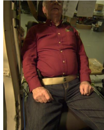
M5-1 Lap buckled, shoulder belt behind seat.
