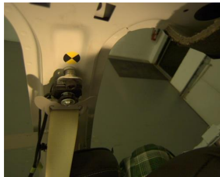
M5-1 Lap buckled, shoulder belt behind seat.
