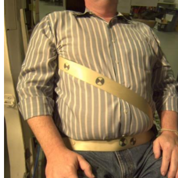
M4-2 Lap buckled, shoulder belt under arm.
