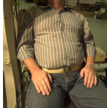
M5-1 Lap buckled, shoulder belt behind seat.
