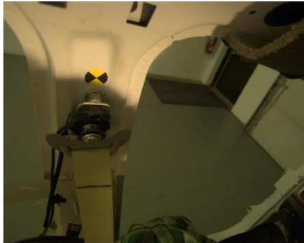
M4-1 Lap buckled, shoulder belt behind back.
