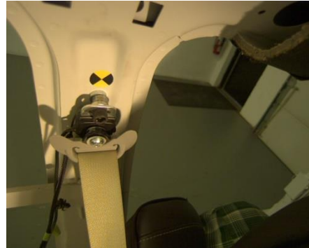
M5-1 Lap buckled, shoulder belt behind seat.
