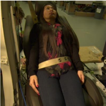
M4-1 Lap buckled, shoulder belt behind back.
