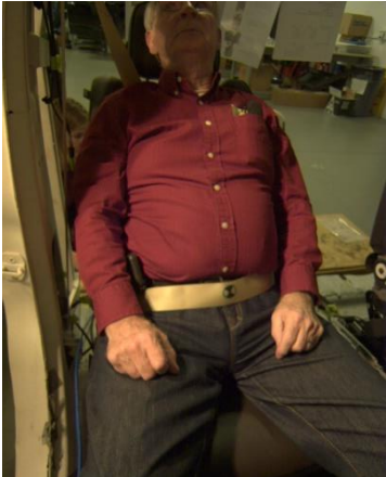
M4-1 Lap buckled, shoulder belt behind back.
