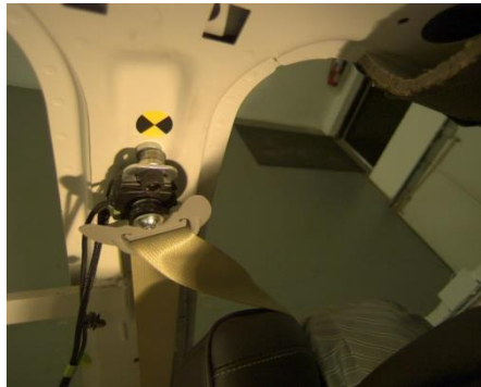
M4-2 Lap buckled, shoulder belt under arm.
