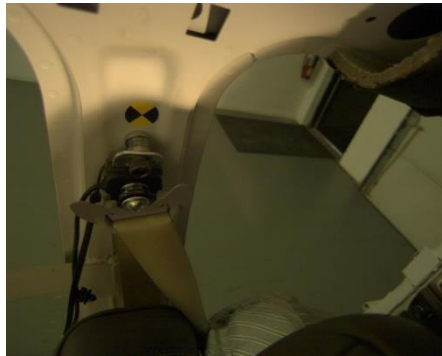
M4-2 Lap buckled shoulder belt under arm.
