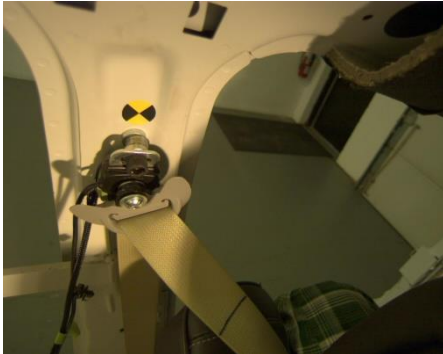
M4-1 Lap buckled, shoulder belt behind back.
