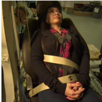
M4-2 Lap buckled, shoulder belt under arm.
