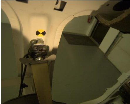
M4-1 Lap buckled, shoulder belt behind back.
