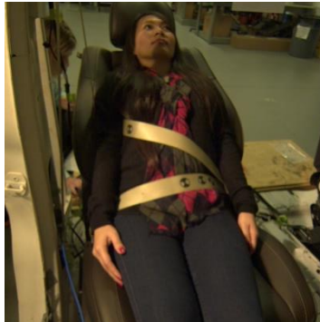
M4-2 Lap buckled, shoulder belt under arm.
