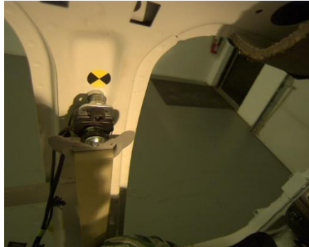
M4-2 Lap buckled, shoulder belt under arm.
