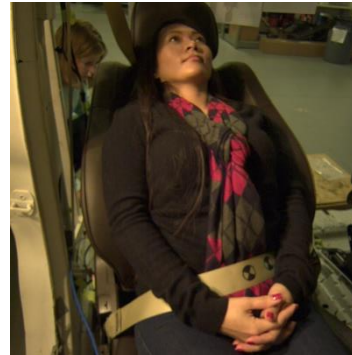
M5-1 Lap buckled, shoulder belt behind seat.
