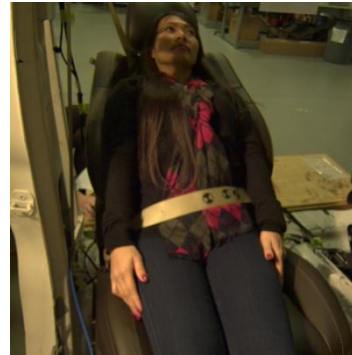
M5-1 Lap buckled, shoulder belt behind seat.
