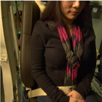
M4-1 Lap buckled, shoulder belt behind back.
