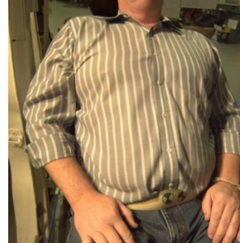
M5-1 Lap buckled, shoulder belt behind seat.
