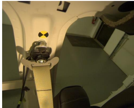
M5-1 Lap buckled, shoulder belt behind seat.
