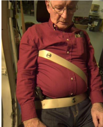
M4-2 Lap buckled, shoulder belt under arm.
