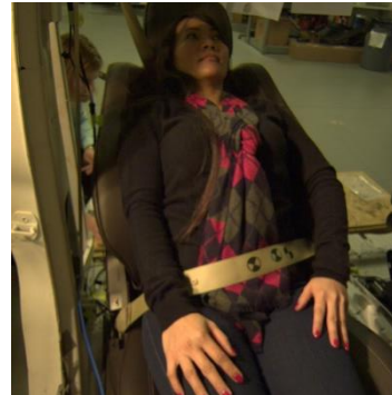
M5-1 Lap buckled, shoulder belt behind seat.
