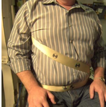
M4-2 Lap buckled, shoulder belt under arm.
