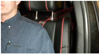
Remove headrest, bring latch plate behind seat through headrest opening and buckle from behind. Occupant buckled.
