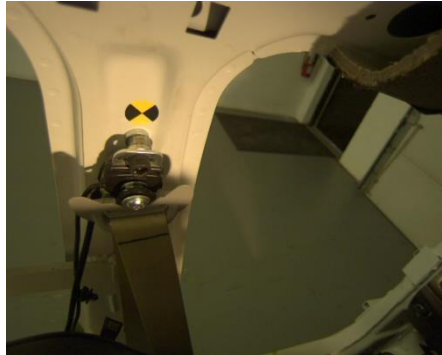
M4-2 Lap buckled, shoulder belt under arm.
