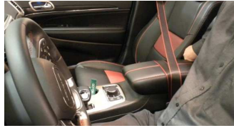
Passenger seat belt latch plate engaged with driver's buckle.
