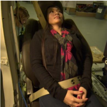
M4-1 Lap buckled, shoulder belt behind back.
