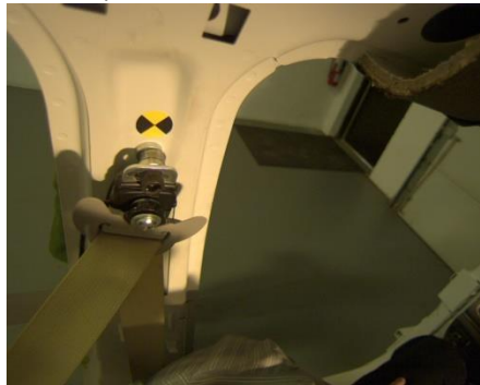
M5-1 Lap buckled, shoulder belt behind seat.
