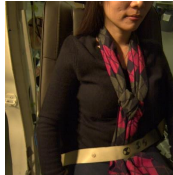
M5-1 Lap buckled, shoulder belt behind seat.
