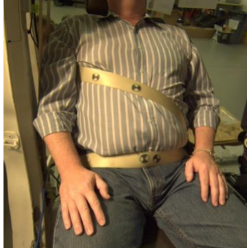
M4-2 Lap buckled, shoulder belt under arm.
