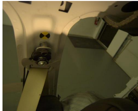
M5-1 Lap buckled, shoulder belt behind seat.
