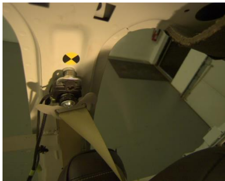
M4-1 Lap buckled shoulder belt behind back.
