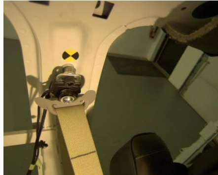
M5-1 Lap buckled, shoulder belt behind seat.
