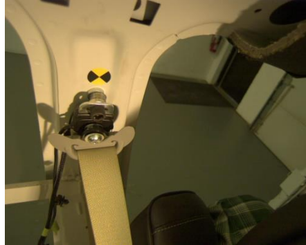
M5-1 Lap buckled, shoulder belt behind seat.
