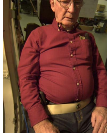
M5-1 Lap buckled, shoulder belt behind seat.
