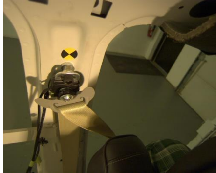
M4-2 Lap buckled, shoulder belt under arm.
