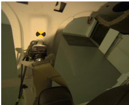
M4-2 Lap buckled shoulder belt under arm.
