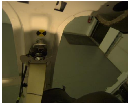
M5-1 Lap buckled, shoulder belt behind seat.
