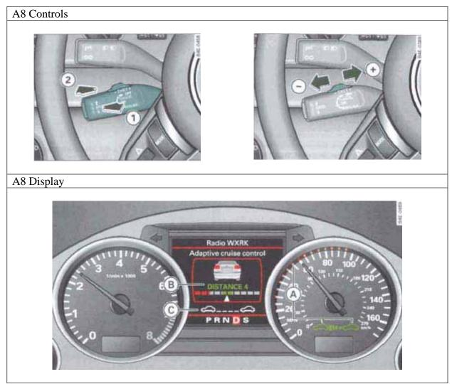
Figure A-1: Audi A8 Adaptive Cruise Control interface elements
