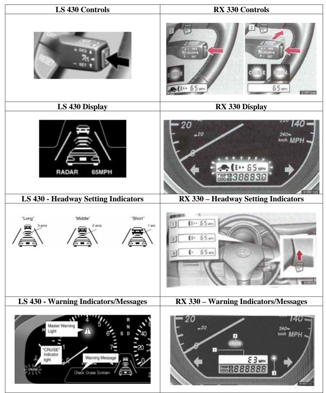
Figure A-7: Lexus Dynamic Laser Cruise Control interface elements
