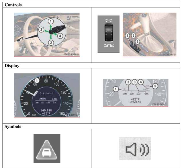
Figure A-8: Mercedes-Benz CLS-class Distronic interface elements
