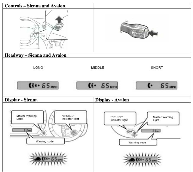
Figure A-9: Toyota Dynamic Laser Cruise Control interface elements
