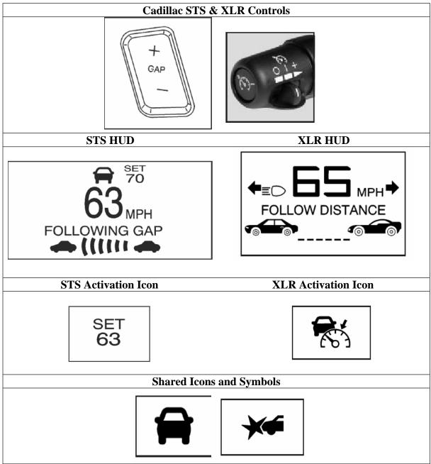
Figure A-3: Cadillac Adaptive Cruise Control interface elements
