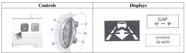
Figure A-6: Jaguar XK Adaptive Cruise Control interface elements
