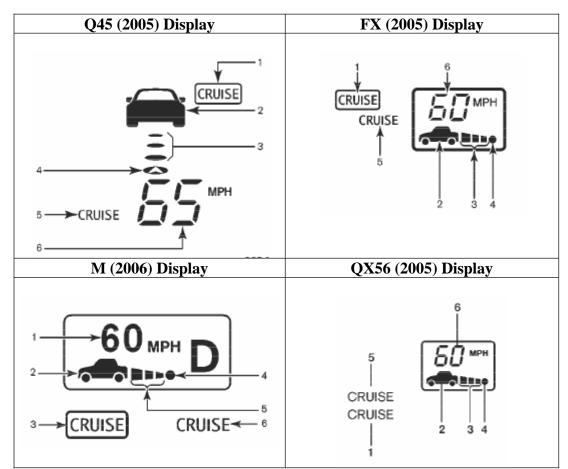
Figure A-5: Infinity Intelligent Cruise Control interface displays
