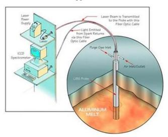
Figure B.33 Schematic of the LIBS ApparatusB
