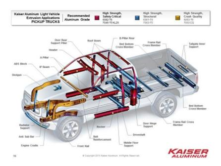
Figure B.24 Kaiser Aluminum Light Vehicle Extrusion Applications in Pickup Trucks<sup>63</sup>
