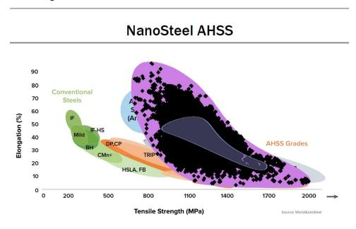
Figure B.17 Comparisons of Established Steel Grades and Potential Nanosteel Grades (in purple)<sup>44</sup>
