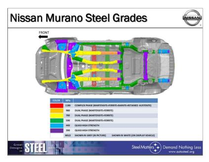
Figure B.15 Nissan Murano Steel Grades for IIHS Compliance - Bottom View<sup>40</sup>
