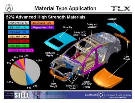
Figure B.7 Material Type Application for the Acura TLX Presented at 2015 Great Designs in Steel<sup>25</sup>
