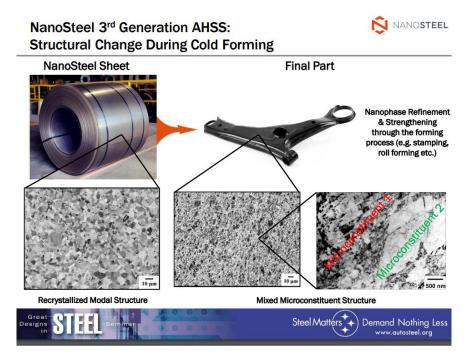
Figure B.18 NanoSteel 3rd Generation AHSS: Structural Change During Cold Forming<sup>44</sup>
