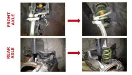
Figure B.44 Glass Fiber Reinforced Polymer Springs (Right) Are A Drop In Replacement For Steel Suspension Springs (Left)<sup>98</sup>
