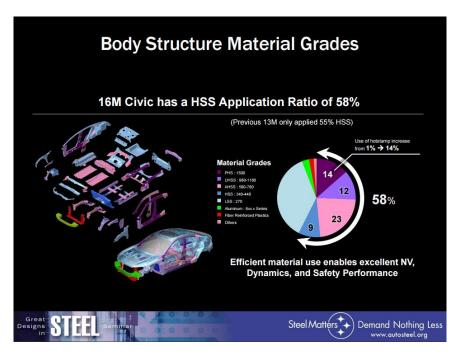
Figure B.8 Body Structure Material Grades for 2016 Honda Civic<sup>29</sup>
