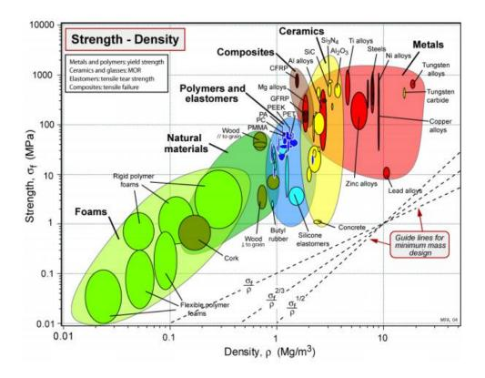
Figure B.1 Ashby Plot for Material Strength-Density<sup>7</sup>
