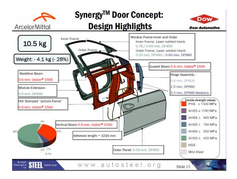
Figure B.4 Arcelor Mittal's Synergy Door Concept Design Highlights 15
