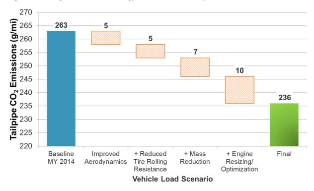
Figure A.1 Potential Reduction in CO<sub>2</sub> Emissions by Adoption of Best-In-Class MY2014 Technologies
