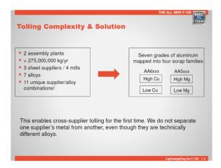
Figure B.36 Coordinating Aluminum Material Recycling 5xxx and 6xxx Grades
