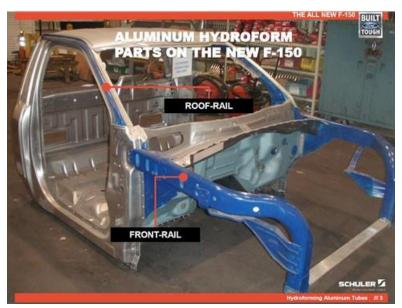
Figure B.26 Aluminum Hydroform Parts on the F-150<sup>64</sup>
