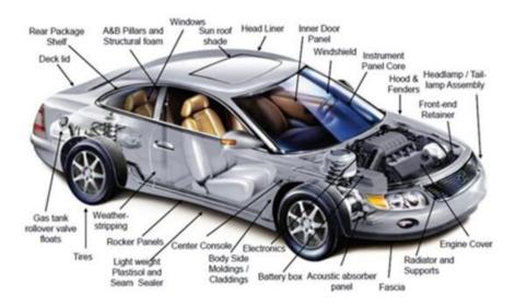
FIGURE 6.2 Auto part targets for lightweight plastics and rubber. Illustration provided by 3M Company.
