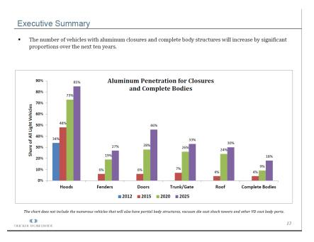
Figure B.20 Ducker Worldwide on Aluminum Penetration for Closures and Complete Bodies
