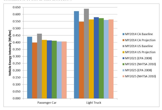
Figure A.2 Sales-Weighted Vehicle Energy Intensity
