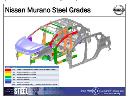
Figure B.14 Nissan Murano Steel Grades used in IIHS Compliance - 3D View<sup>40</sup>
