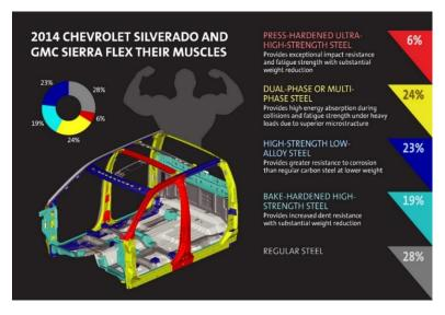
Figure B.9 High Strength and Ultra High Strength Steel changes in the 2014 Silverado 1500<sup>30</sup>
