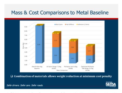
Figure B.54 Mass and Cost Comparisons of Composite Fiber B Pillar to Metal Baseline
