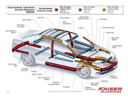
Figure B.25 Kaiser Aluminum Light Vehicle Extrusion Applications in Sedans<sup>63</sup>
