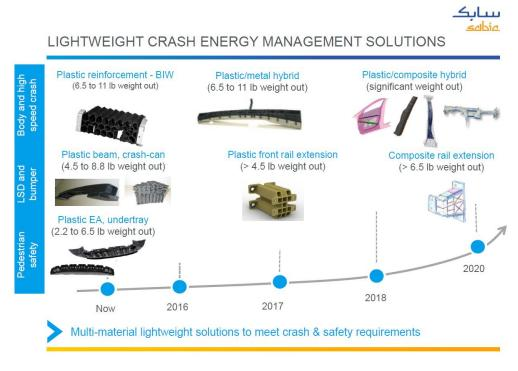
Figure B.47 SABIC Potential Lightweight Crash Energy Management Solutions<sup>111</sup>
