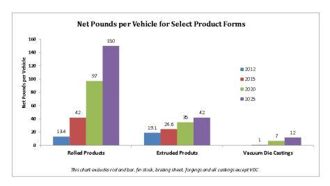
Figure B.21 Ducker Worldwide Estimates of Rolled, Extruded and Vacuum Die Cast Aluminum Product Demand Increase
