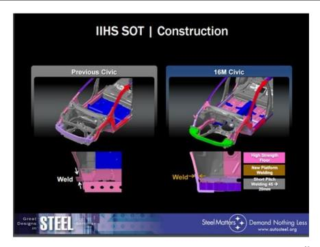
Figure B.16 Honda Civic IIHS Small Overlap Test Construction Upgrades<sup>29</sup>
