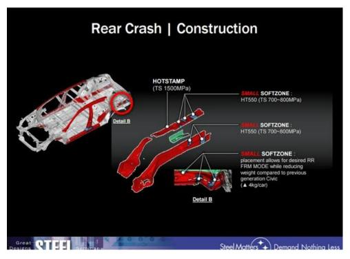
Figure B.13 Honda Civic Rear Crash Construction Including Softzones While Reducing Mass<sup>29</sup>
