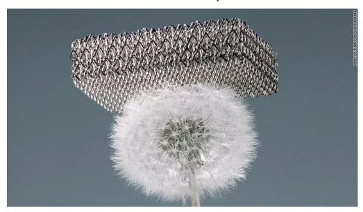
Figure B.19 Microlattice Material by HRL Laboratories
