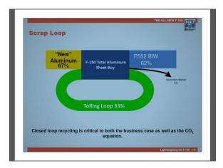
Figure B.35 Scrap Loop - 33% Manufacturing Scrap is Recycled into New Sheet Product and 5% Castings
