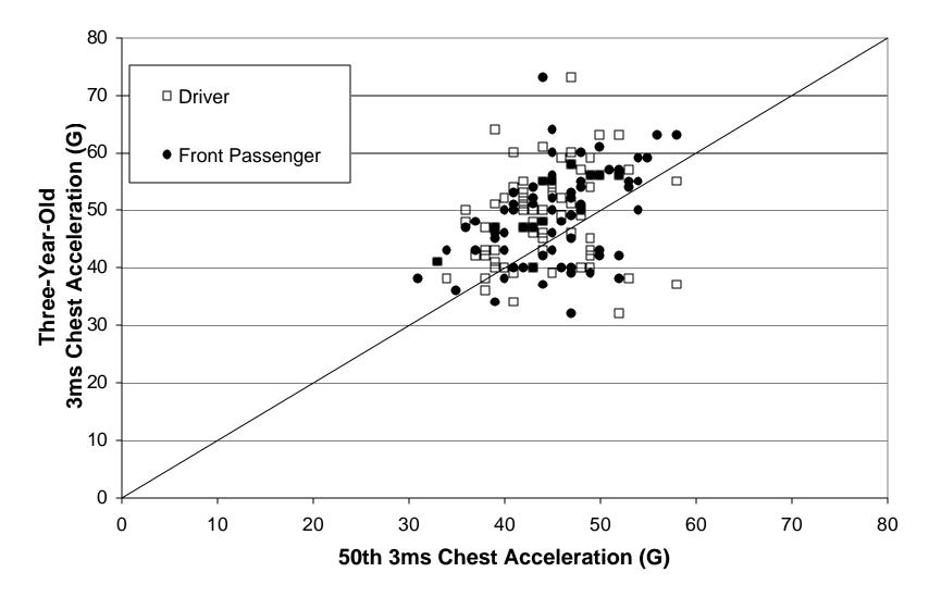
Figure 12: Chest G Comparison Between Three-Year-Old and 50th-percentile
