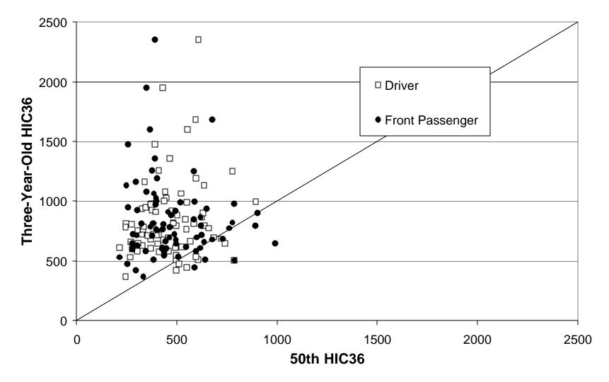
Figure 11: HIC Comparison Between Three-Year-Old and 50th-percentile
