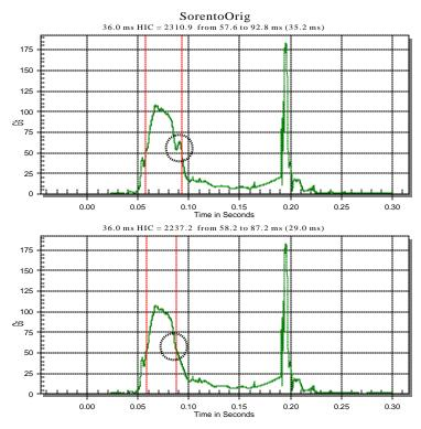
Figure B2: 2003 Kia Sorento 6YO HIC readings, with and without face-to-chest contact
