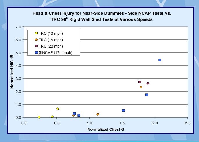
In general, near-side dummy readings for HIC 15 & chest G in 15 mph rigid wall sled tests are similar to readings in SINCAP vehicle tests
