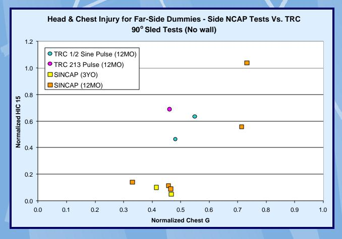
Inconclusive whether HIC 15 & chest G readings for far-side dummy in vehicle tests greater than in sled tests (no wall)
