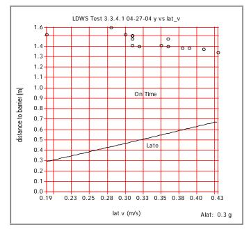
Figure 5. Results from a road-departure toward Jersey barrier test. The plot shows range to the barrier at the time of warning as a function of lateral velocity toward the barrier. All the warnings were on time (i.e., they occurred above the CPB line).
