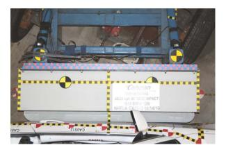
Overhead View of Aligned MDB and Vehicle at Impact Location \_\_8
