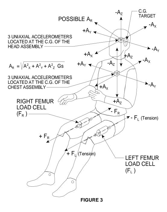
TABLE 2. SIGN CONVENTION FOR HYBRID III TRANSDUCER OUTPUTS
