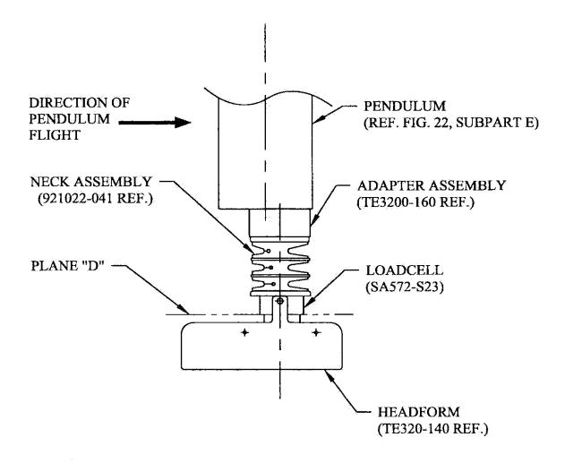
NOTE: MOUNT NECK AT LEADING EDGE OF PENDULUM TO AVOID INTERFERENCE.
