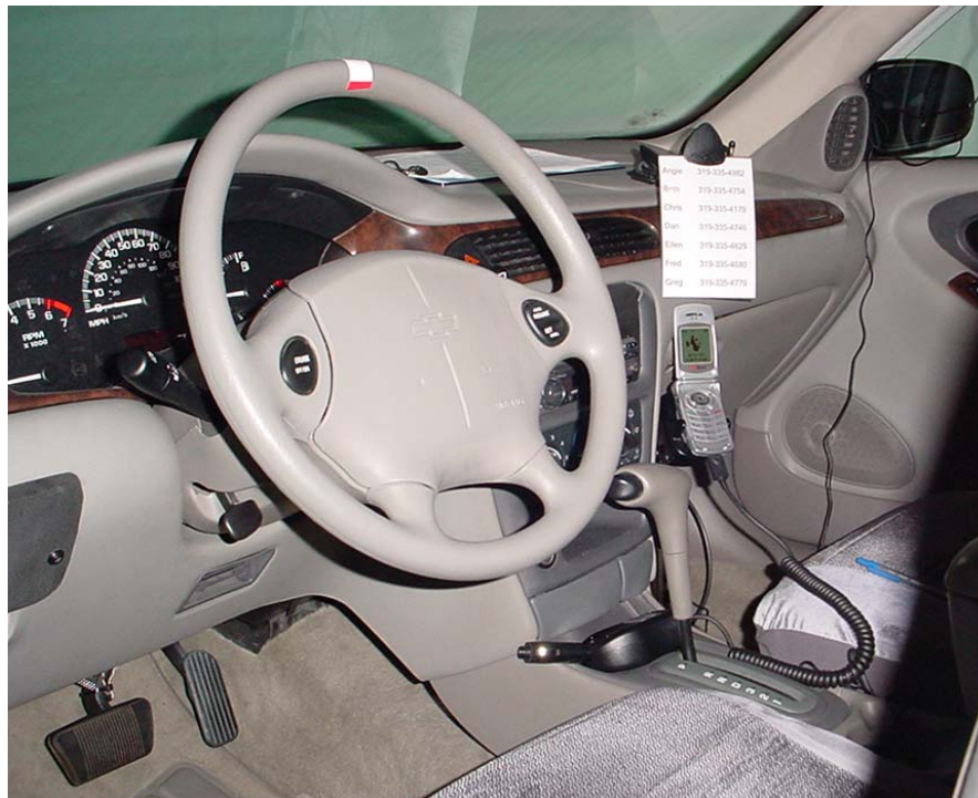
Figure 14. Photograph Showing Location of Phone Cradle and Phone Number Pad Location.
