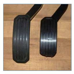
Figure 36 – Modified Pedals (NHTSA Recall 09V388/Toyota Recall 90L)
