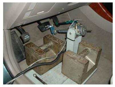
Figure 5 - Setup of Brake Pedal Force versus Displacement Device in a Typical Test Vehicle
