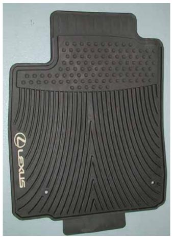
Figure 33 - Floor Mat Design Used to Evaluate Potential for Pedal Entrapment Test
