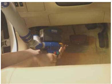
Figure 8 - FARO Laser Scan Arm Operating in Vehicle
