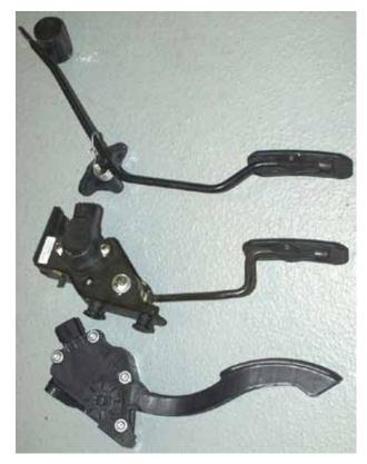
Figure 24 – Three Pedal Generations, Cable driven (top), Potentiometer (center), Hall Effect (bottom)
