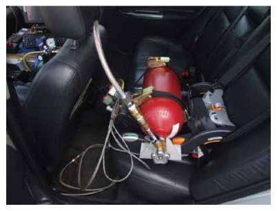
Figure 4 - Nitrogen Supply Tank and Solenoid Valves Used for Pneumatic Brake Ram Actuation
