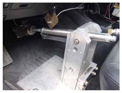
Figure 3 - Pneumatic Brake Ram Used in Testing
