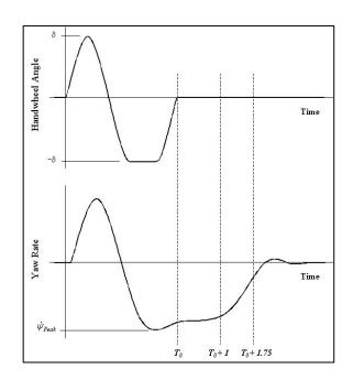
Figure 4. Steering wheel position and yaw velocity information used to assess lateral stability.
