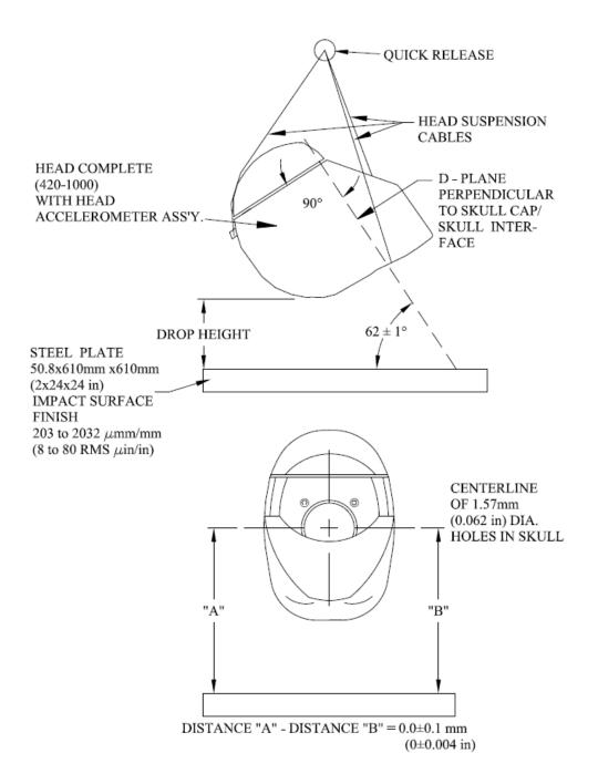
FIGURE T2 NECK FLEXION TEST SET-UP SPECIFICATIONS
