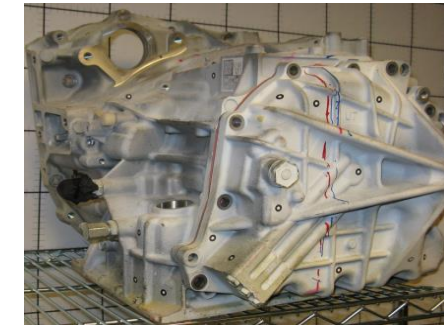
Case Subsystem-Replace with a 390 Aluminum casting with Mg AJ62 (Mg-Al-Sr)
