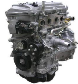
Venza Base Engine (Toyota 2.7L 1AR-FE) Engine Downsize Selection (Toyota 2.4L 2AZ-FE)
