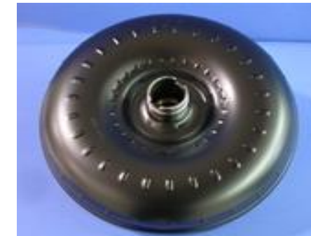
Launch Clutch Subsystem-Replace steel torque converter with Aluminum
