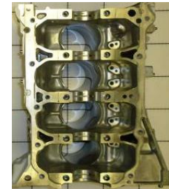
Baseline--Die cast aluminum engine block with cast iron cylinder liners New Design--Magnesium Aluminum Hybrid Engine Block with plasma cylinder liner
