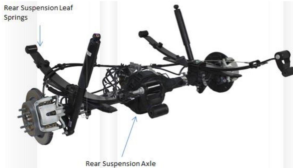
Figure 554: Ford F150 Rear Axle / Suspension 216
