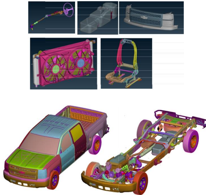
Figure 288: Baseline Vehicle LSDYNA FEA Model Details
