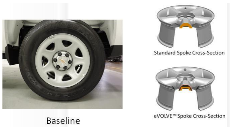
Figure 478: Baseline Wheels vs. LWT Wheels
