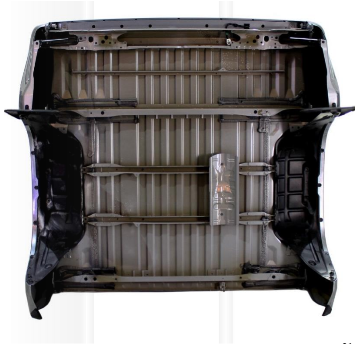
Figure 551: Toyota Tundra Pickup Box Underside 214
