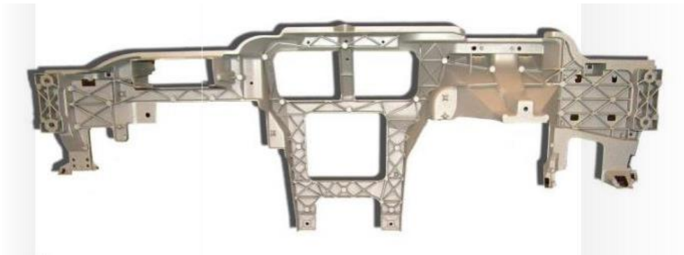
Figure 240: BMW E70 Cast Magnesium I/P Beam
