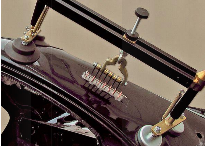
Figure 397: Typical Dent Puller Frame
