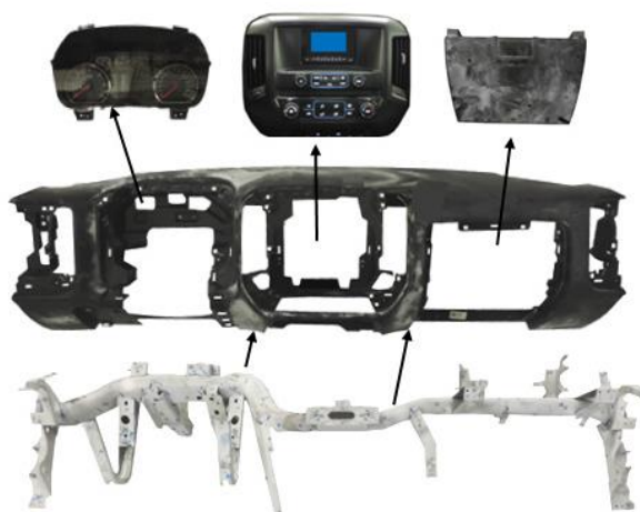
Figure 37: Instrument Panel Components
