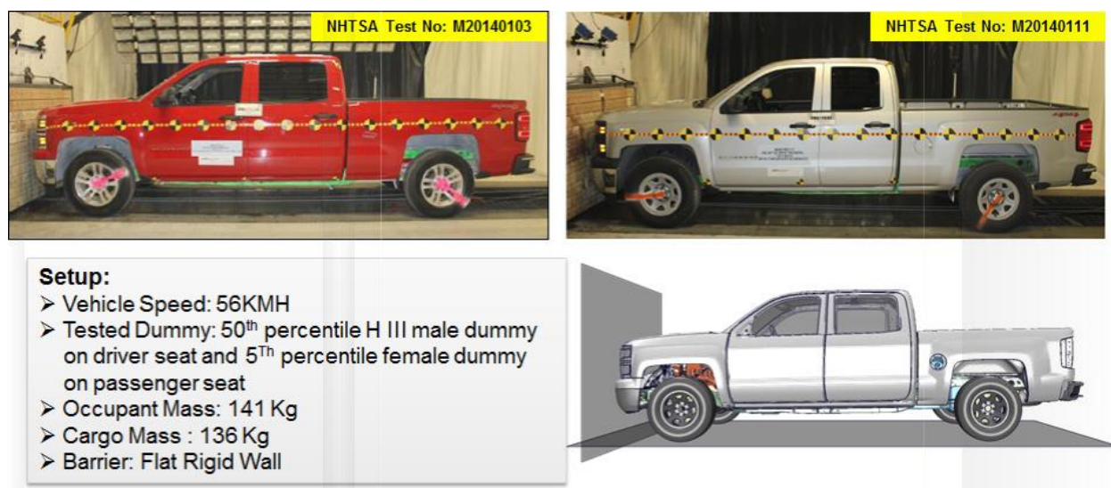
Figure 306: NCAP Frontal - Test and LS-DYNA Model set up
