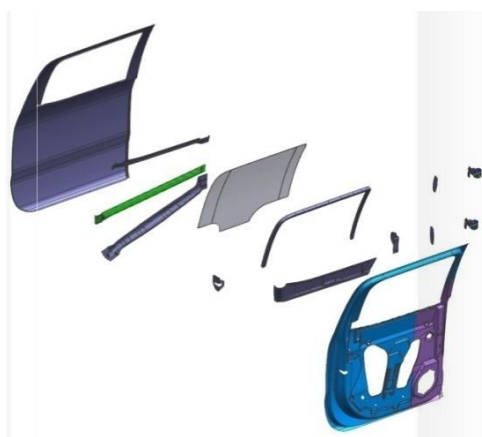
Figure 167: Baseline Rear Door Exploded View
