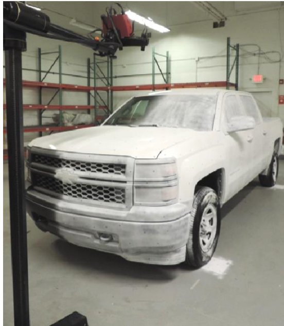
Figure 16: Silverado 1500 Exterior Prepared for White Light Scanning
