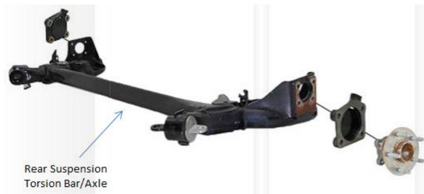
Figure 530: Chevrolet Sonic rear suspension 200
