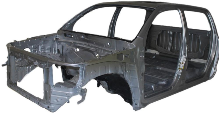
Figure 550: Toyota Tundra Cab Structure 213
