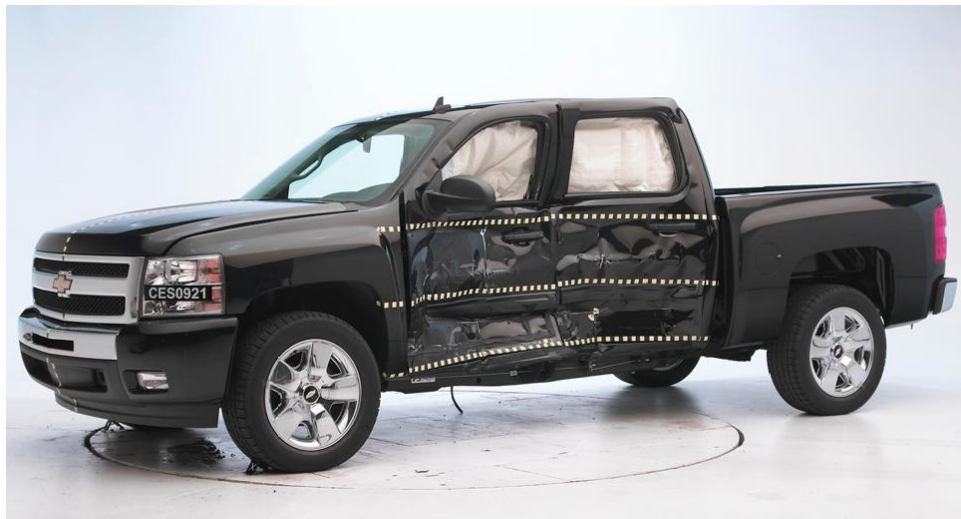
Figure 89: 2010 Chevrolet Silverado 1500 Following IIHS Side Impact Test
