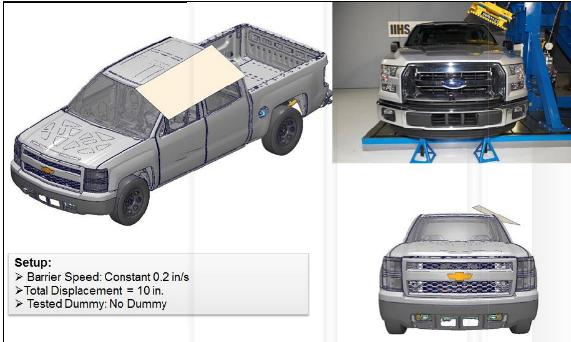
Figure 331: IIHS Roof Strength Test - LS-DYNA Model Setup
