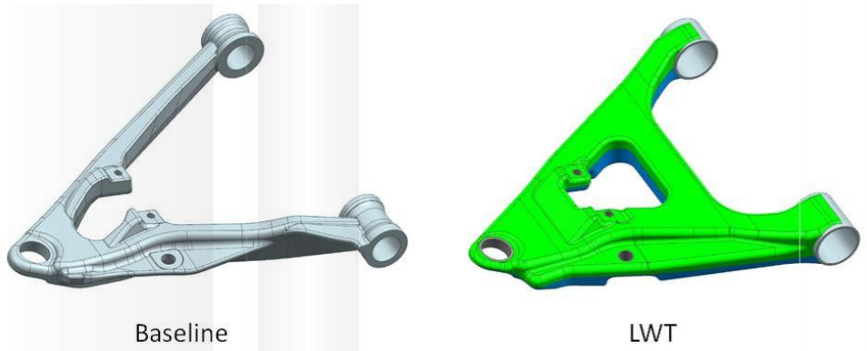
Figure 473: Lower Control Arm – Baseline vs. LWT
