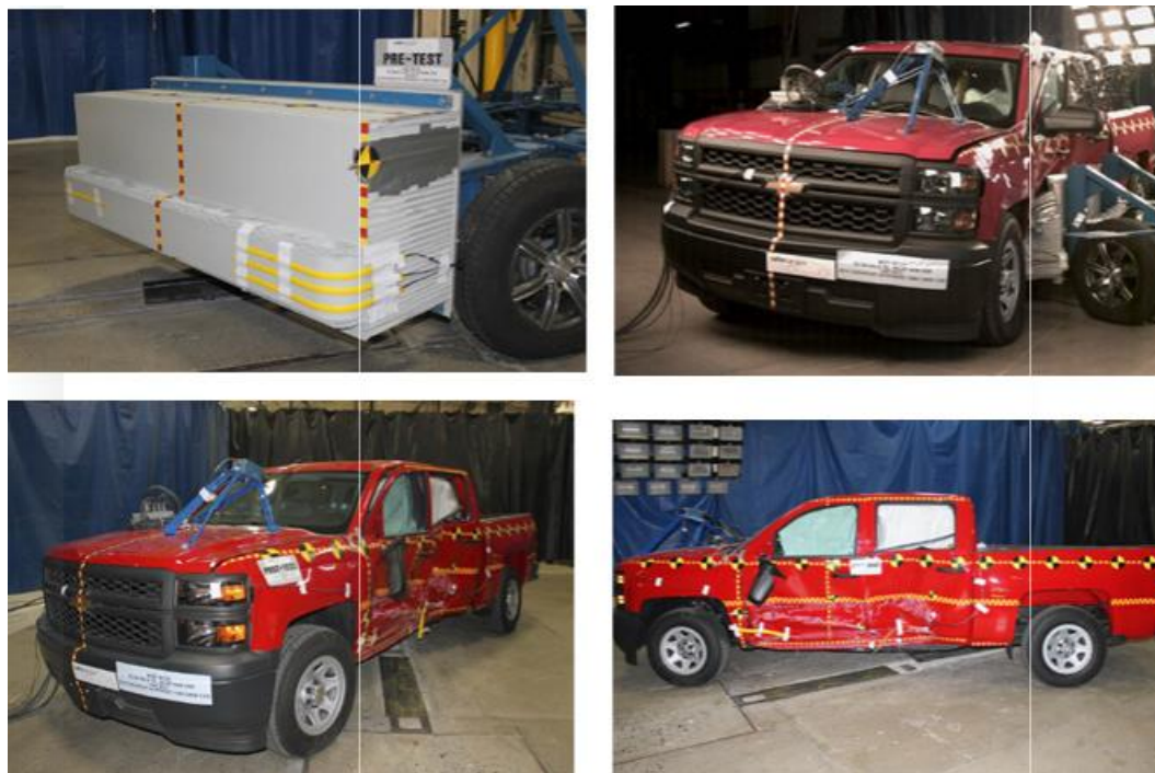
Figure 71: MDB and Post-Test Vehicle following 2014 Silverado 1500 NC P Side Impact Test with MDB
