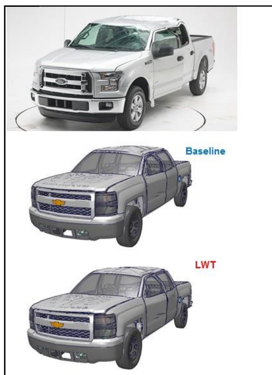
Figure 332: IIHS Roof Strength Test - Comparison Test v Baseline and LWT
