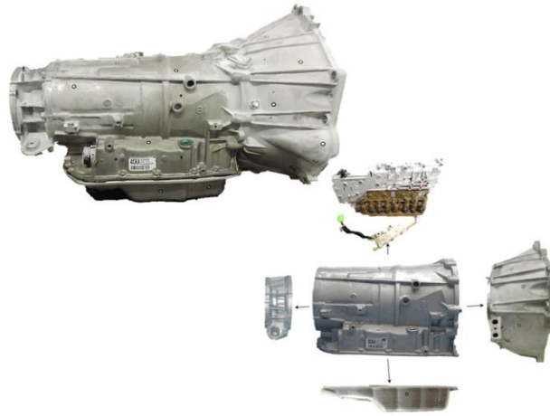
Figure 53: Transmission Assembly
