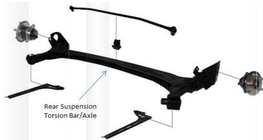
Figure 533: Toyota Corolla rear suspension 202
