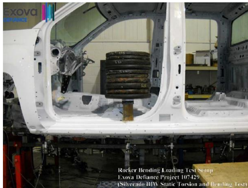
Figure 110: 2014 Silverado Sill Loaded Bending Test
