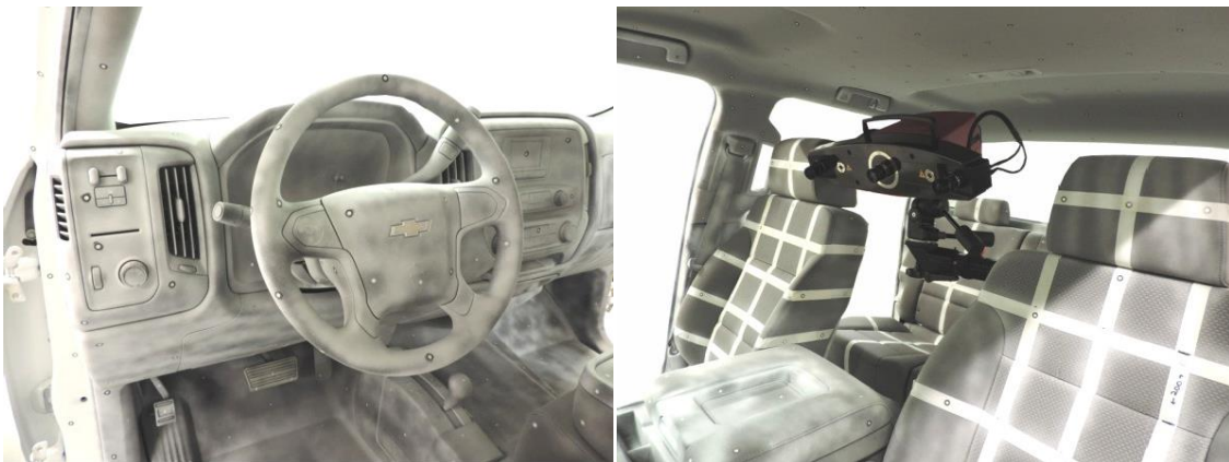
Figure 17: Silverado 1500 Interior Prepared for White Light Scanning
