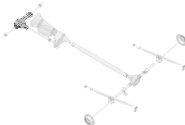
Figure 225: Front Differential
