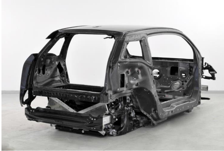
Figure 131: 2014 BMW i3 – Composite and Aluminum Structure 94
