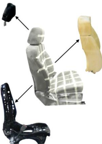
Figure 31: Front Seat Assembly
