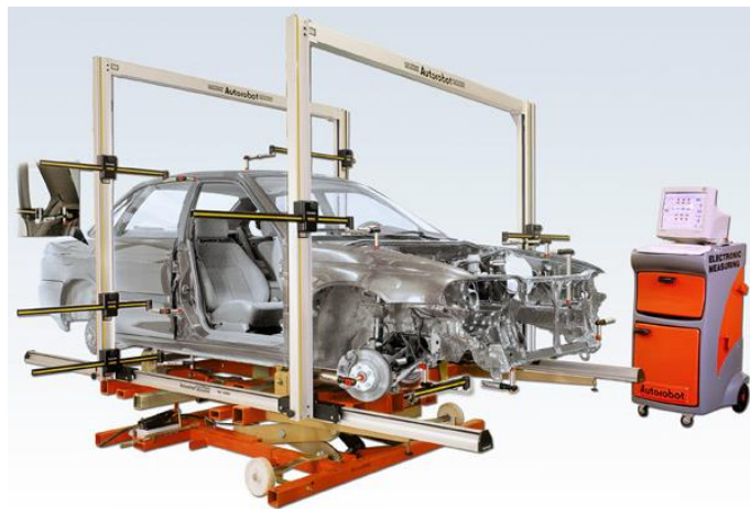
Figure 395: Vehicle on a Typical Dimensional Checking Rig
