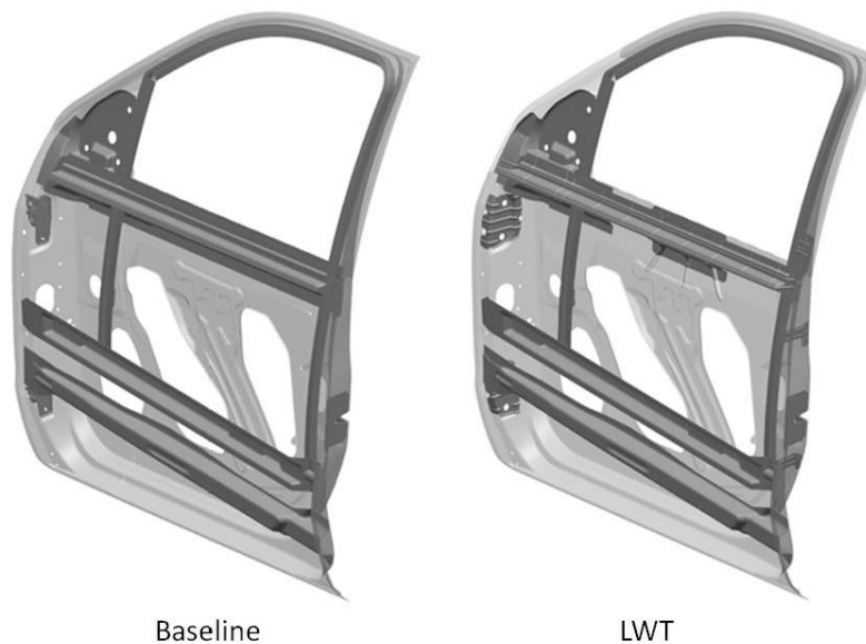
Figure 449: Front Door Frames – Baseline vs. LWT
