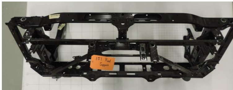
Figure 440: Baseline Chevrolet Silverado Radiator Support Assembly
