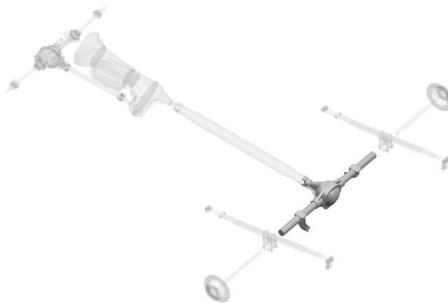
Figure 226: Rear Axle / Differential
