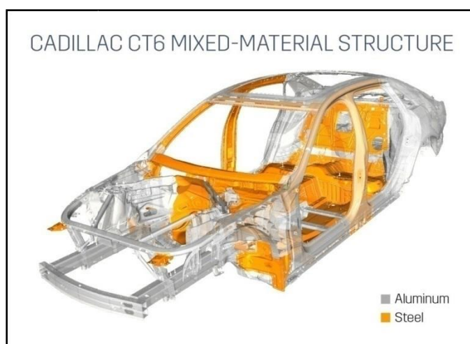
Figure 124: 2016 GM Cadillac CT6 Body Structure
