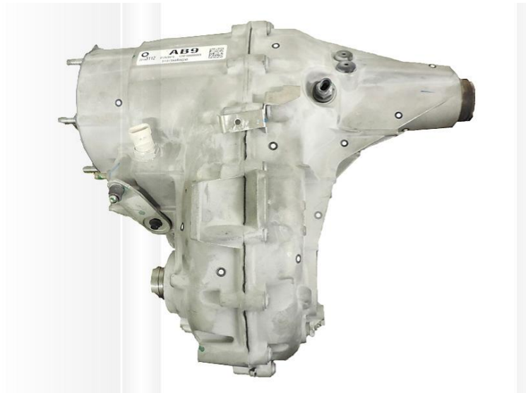
Figure 56: Transfer Case Assembly
