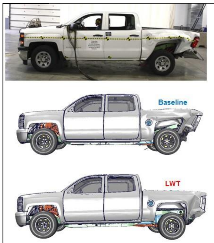
Figure 348: FMVSS 301R - Post-Crash Comparison Between Test and Baseline
