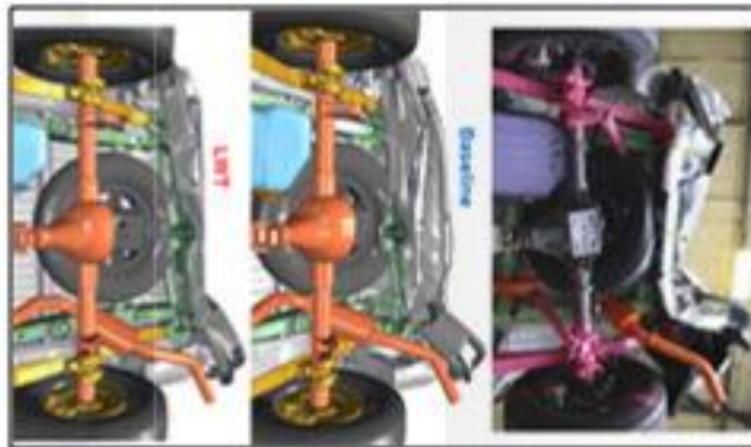
Figure 347: FMVSS 301R - Post-Crash Comparison Between Test and Baseline
