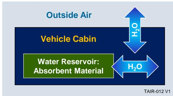
**Figure 11. Moisture Movement in a Vehicle Cabin**
