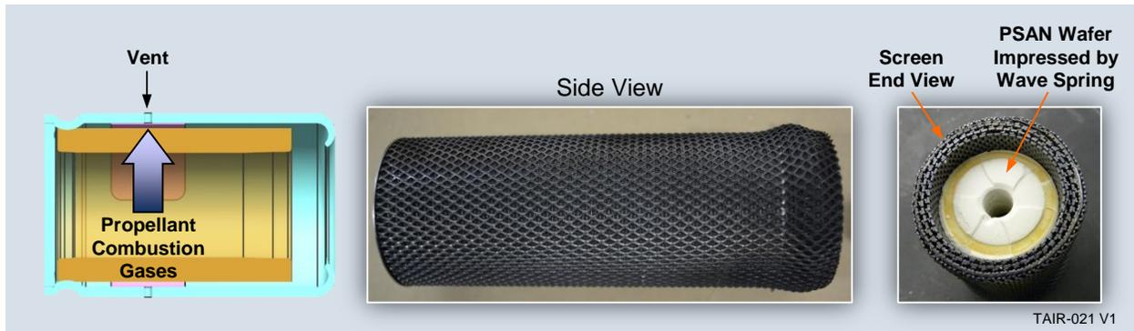
Figure 20. Typical Passenger Cooling Screen
