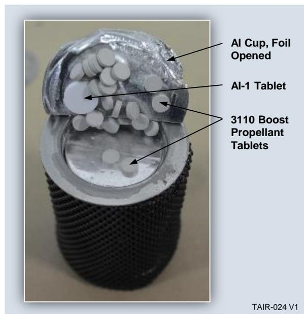
Figure 23. Typical Passenger AI Cup
