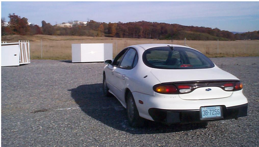
**Figure 10. Subject vehicle parked at an eye distance of 40 feet from the test rig. Discomfort glare was measured at this distance, while attention getting and peripheral detection were measured at an eye distance of 150 feet. Notice the cart with spare mask boards to the left of the test rig.**
