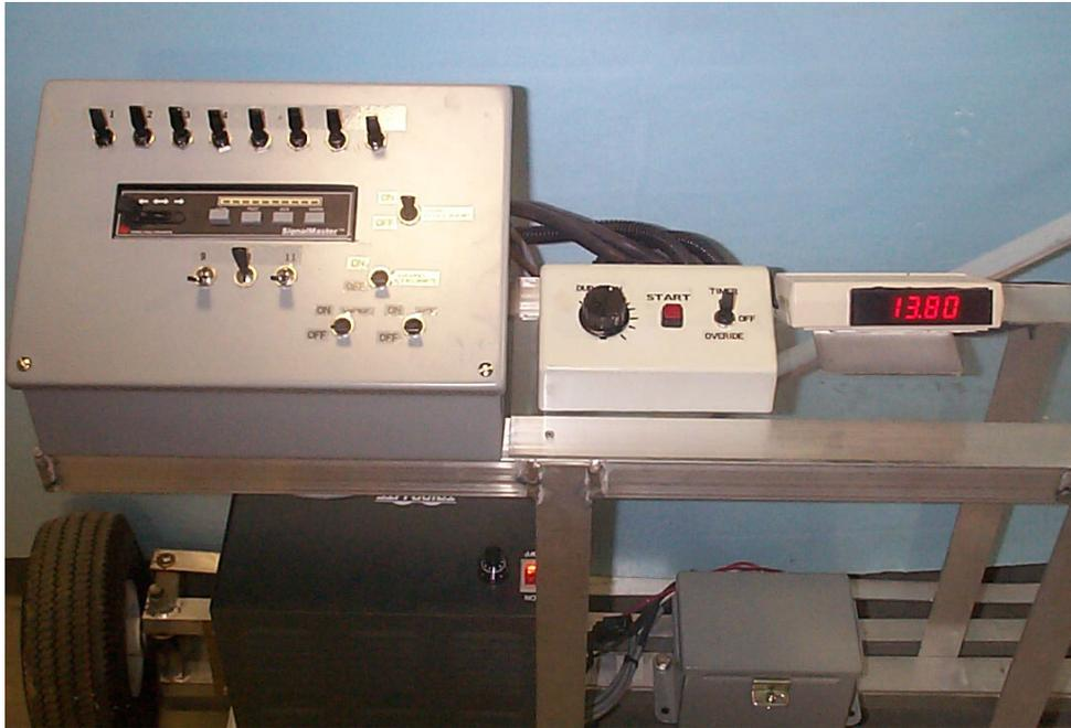
**Figure D3. The control panel for the lighting assembly test rig. The power supply is shown in the bottom left corner, while the light-tight box used for the strobes is in the lower right. The upper left box is the main control panel. In the upper middle is the timer controls for the timed peripheral detection tasks, and in the upper right is the voltmeter which was monitored to assure a consistent power supply.**
