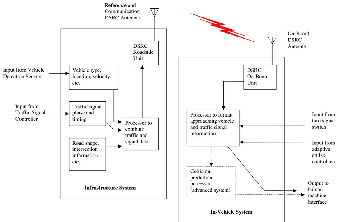
Figure 4.22 Block Diagram of the Left Turn Assistant
