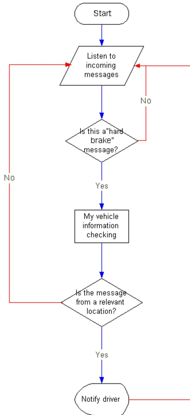
Figure 4.12 Emergency Electronic Brake Light Flow Chart
