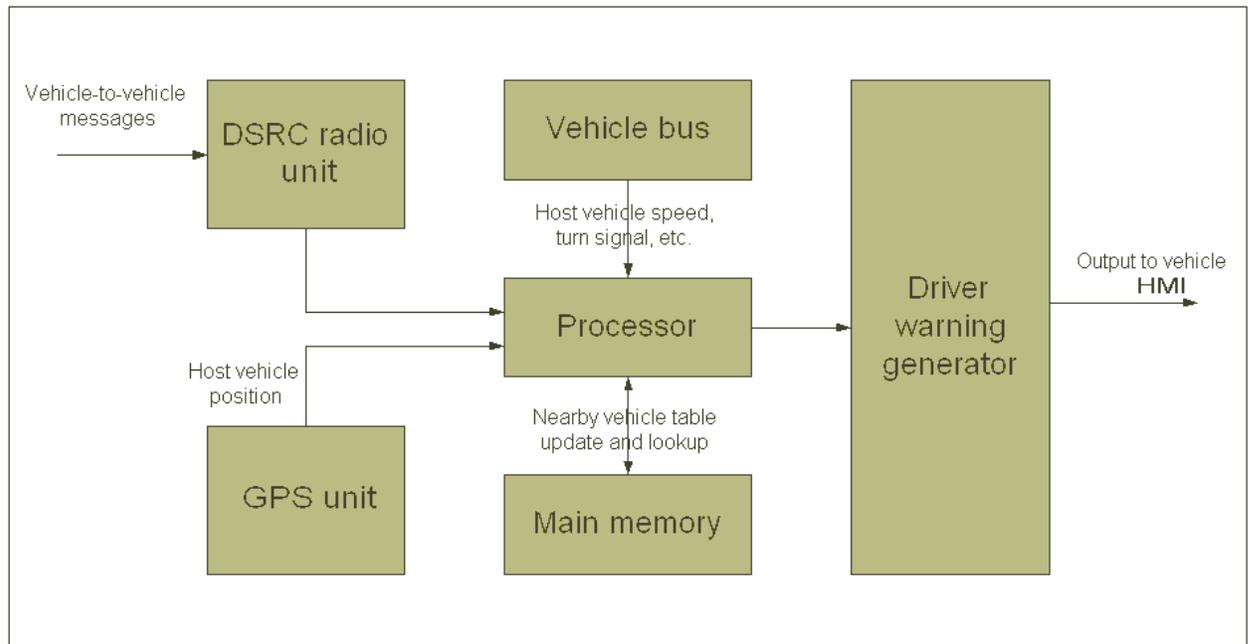
**Figure 4.28 Application Host Vehicle Architecture and Information Flow**
