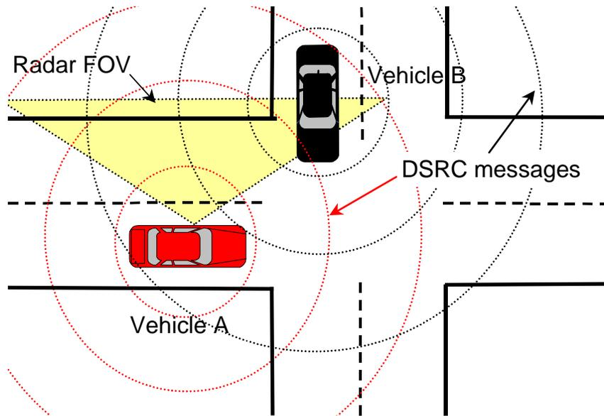
**Figure 4.14 Pre-Crash Sensing for Cooperative Collision Mitigation: Side Impact Scenario**
