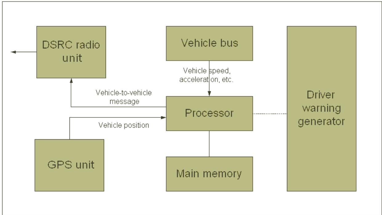
**Figure 4.11 Emergency Electronic Brake Light Block Diagram II**
