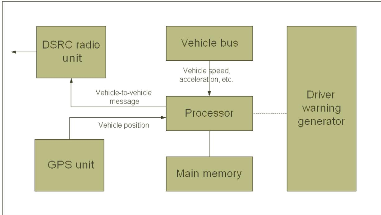
**Figure 4.29 Vehicle-to-Vehicle Message Sender Architecture and Information Flow**
