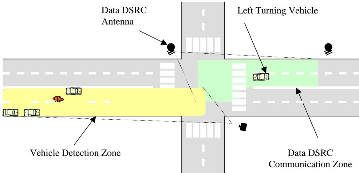
**Figure 4.20 Data DSRC Communications**
