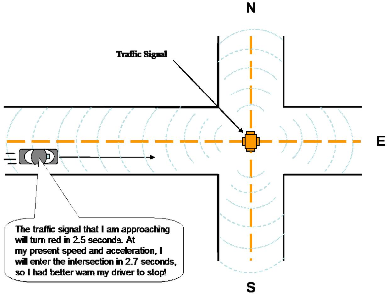
Figure 4.4 Traffic Signal Violation Warning: Vehicle Approaching – Warning Required
