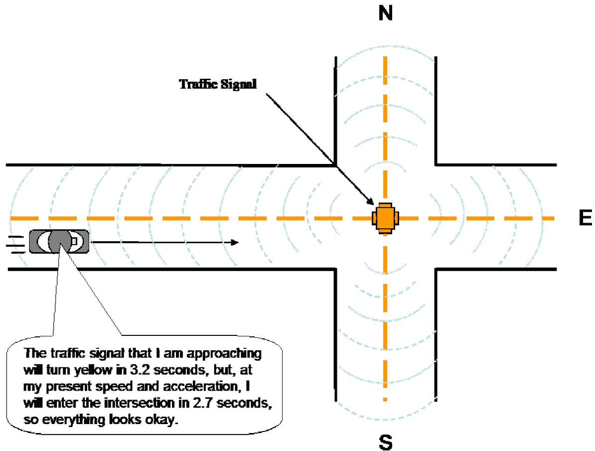
Figure 4.2 Traffic Signal Violation Warning: Vehicle Approaching - Okay to Proceed
