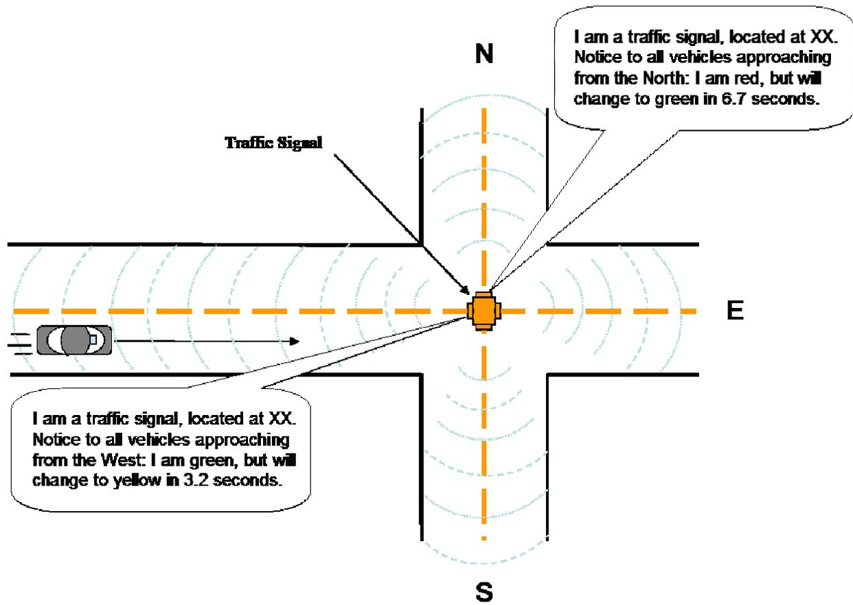
Figure 4.1 Traffic Signal Violation Warning: Directed Signal Phase Messages – Turning Yellow
