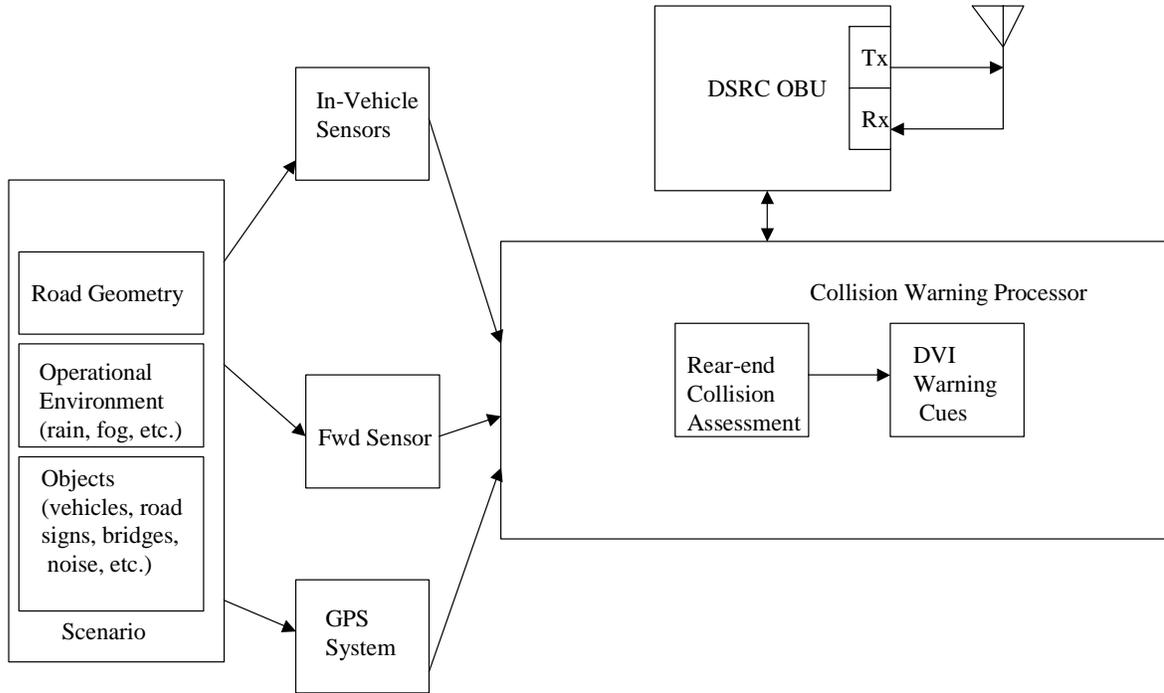
**Figure 4.17 Block Diagram of Cooperative Forward Collision Warning System**
