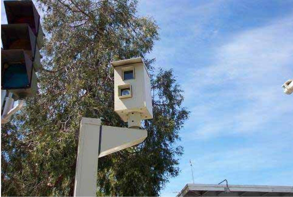
**Figure 23.** Picture of Red Light Photo Enforcement Camera in the City of Sacramento
