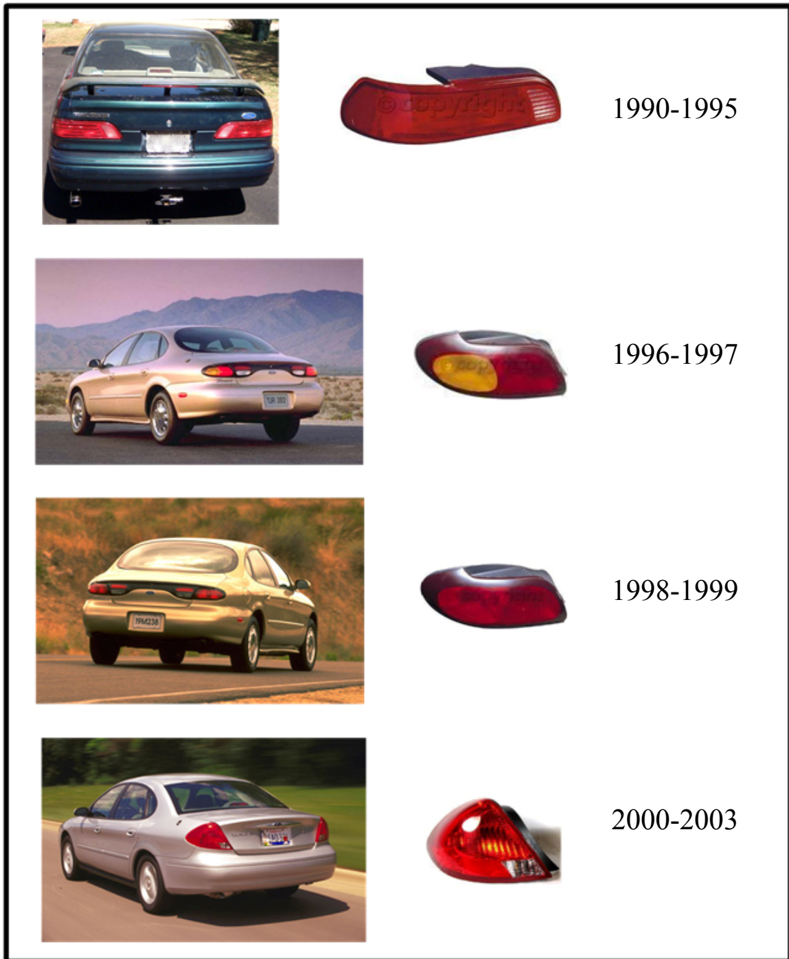
Figure 8. Changes in turn signal color within the Ford Taurus from 1990 to 2003.
