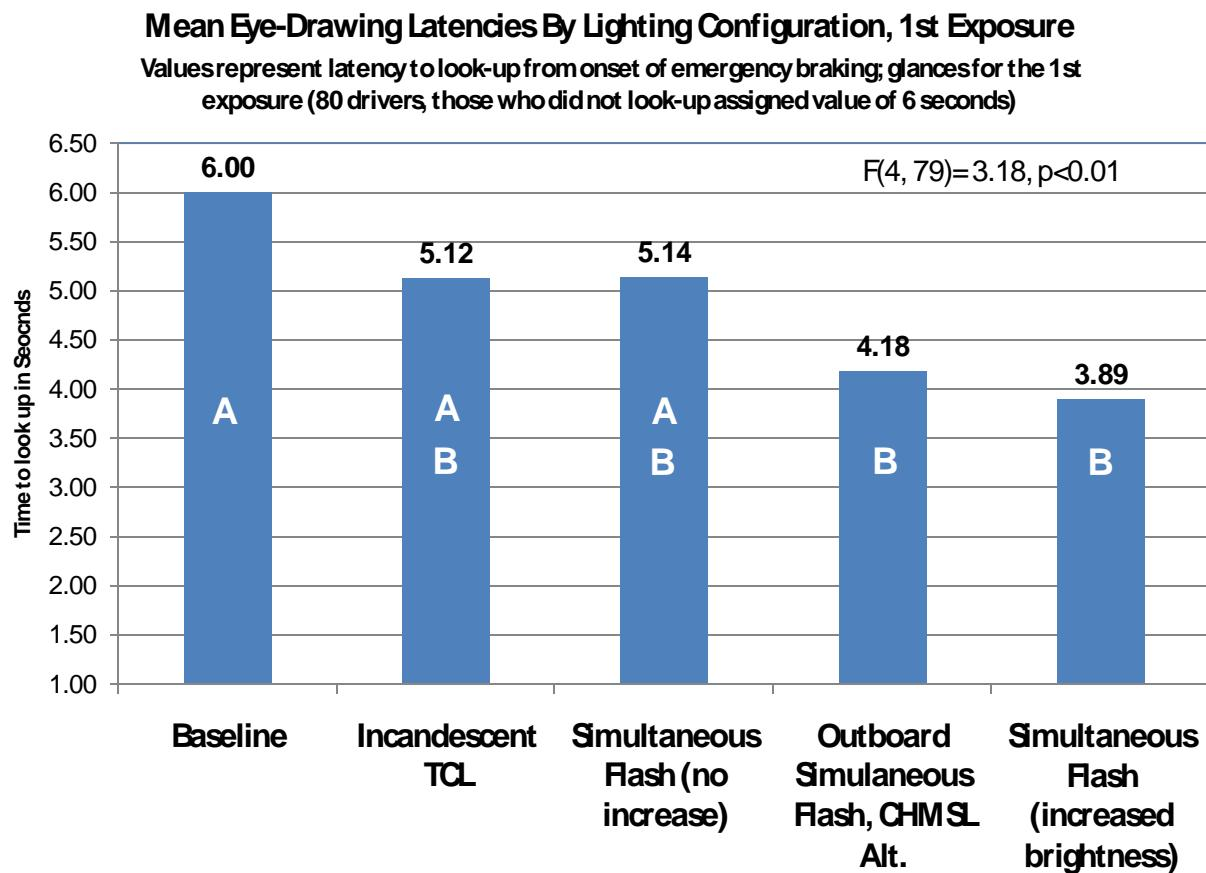
**Figure 23. Mean Look-up Response Times on First Exposure to the Lighting Display as a Function of Lighting Configuration**
