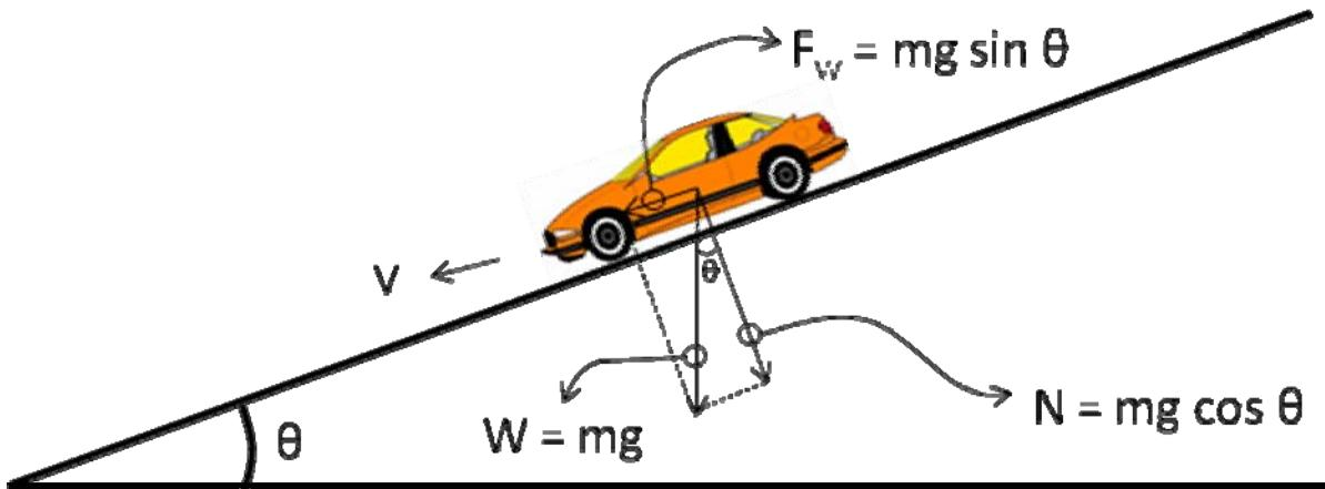
**Figure 56. Forces on a Vehicle Created by a Downward Slope**
