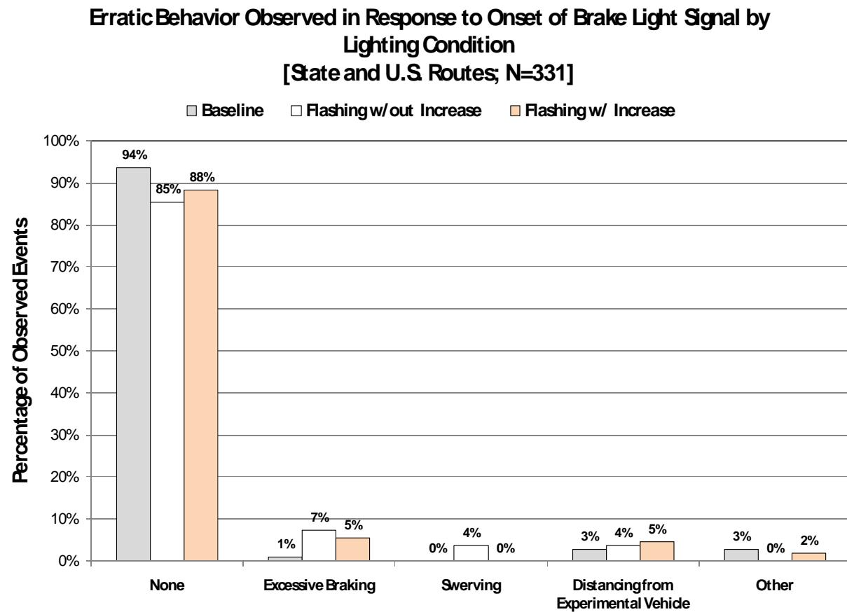
**Figure 53. Incidence of Erratic Behaviors (Pooled State and U.S. Route Car-Following, n=331. Does Not Include Adjacent Vehicle Trials Data.)**
