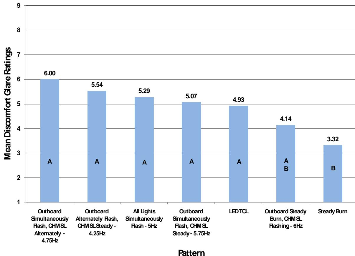
**Figure 15. Results of the Discomfort Glare Ratings at 100 ft (30.5 m) Looking Directly Forward**
