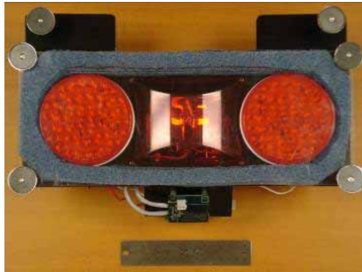
**Figure 20. CHMSL Assembly Including the Center Incandescent TCL With Side LED Lamps**
