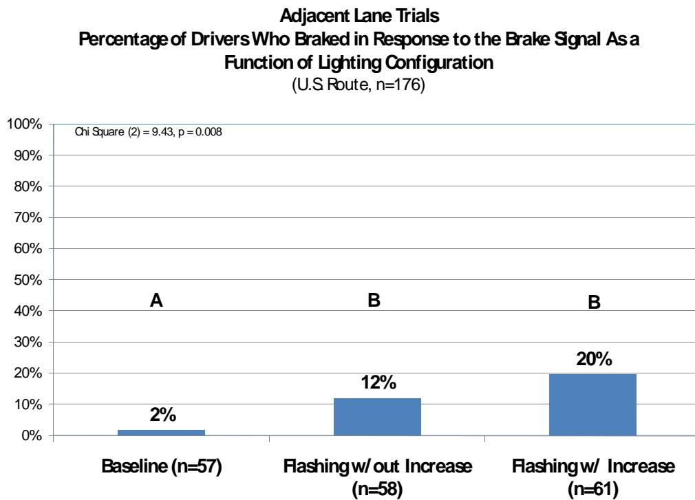
**Figure 52. Percentage of Adjacent Vehicle Drivers Observed to Brake in Response to the Signal (U.S. Route).**
