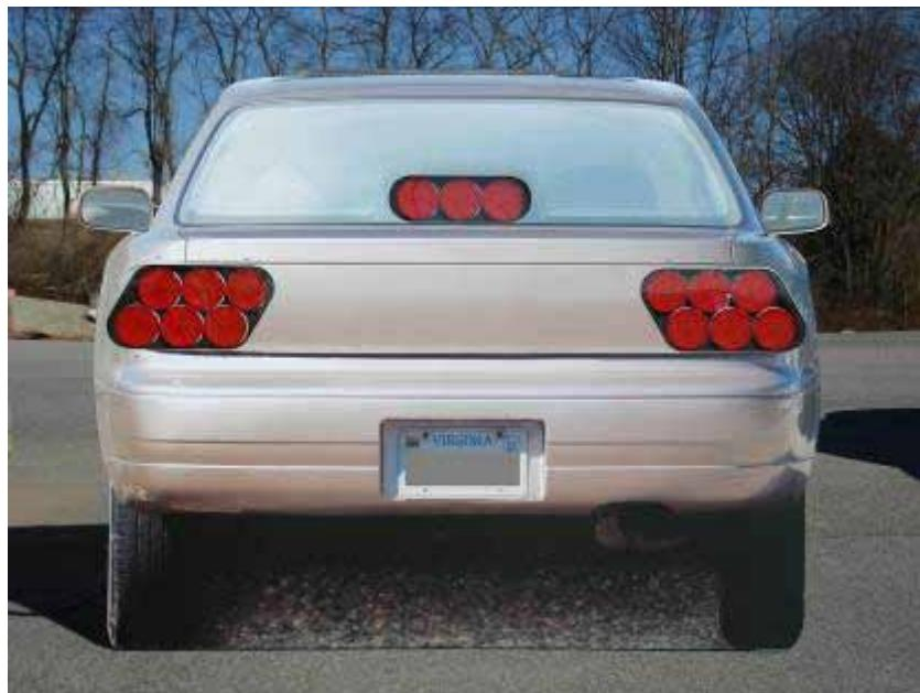
**Figure 21. Vehicle Mock-Up With Working Brake Lamps**
