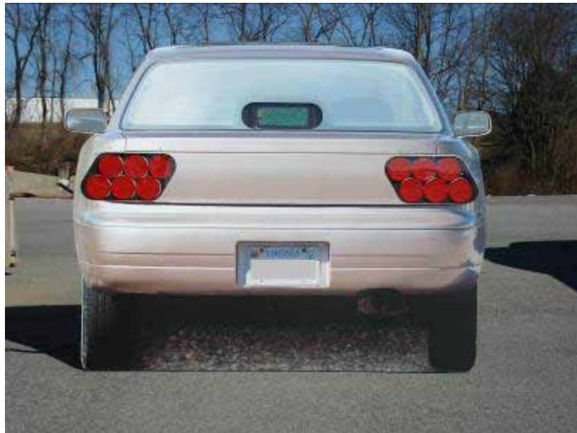
**Figure 7. Test Apparatus Using the LED TCL in the CHMSL Position.**
