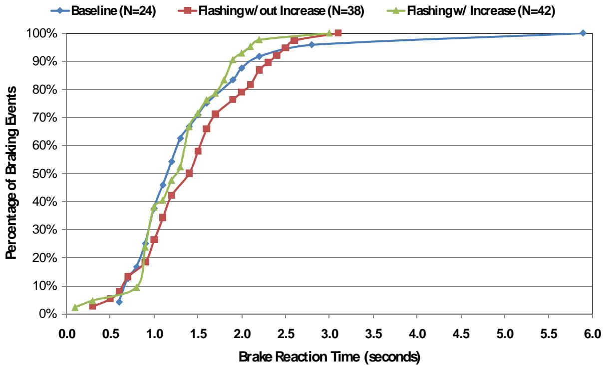
**Figure 50. Cumulative Distribution of Brake Response Times (Pooled for State and U.S. Route Data)**
