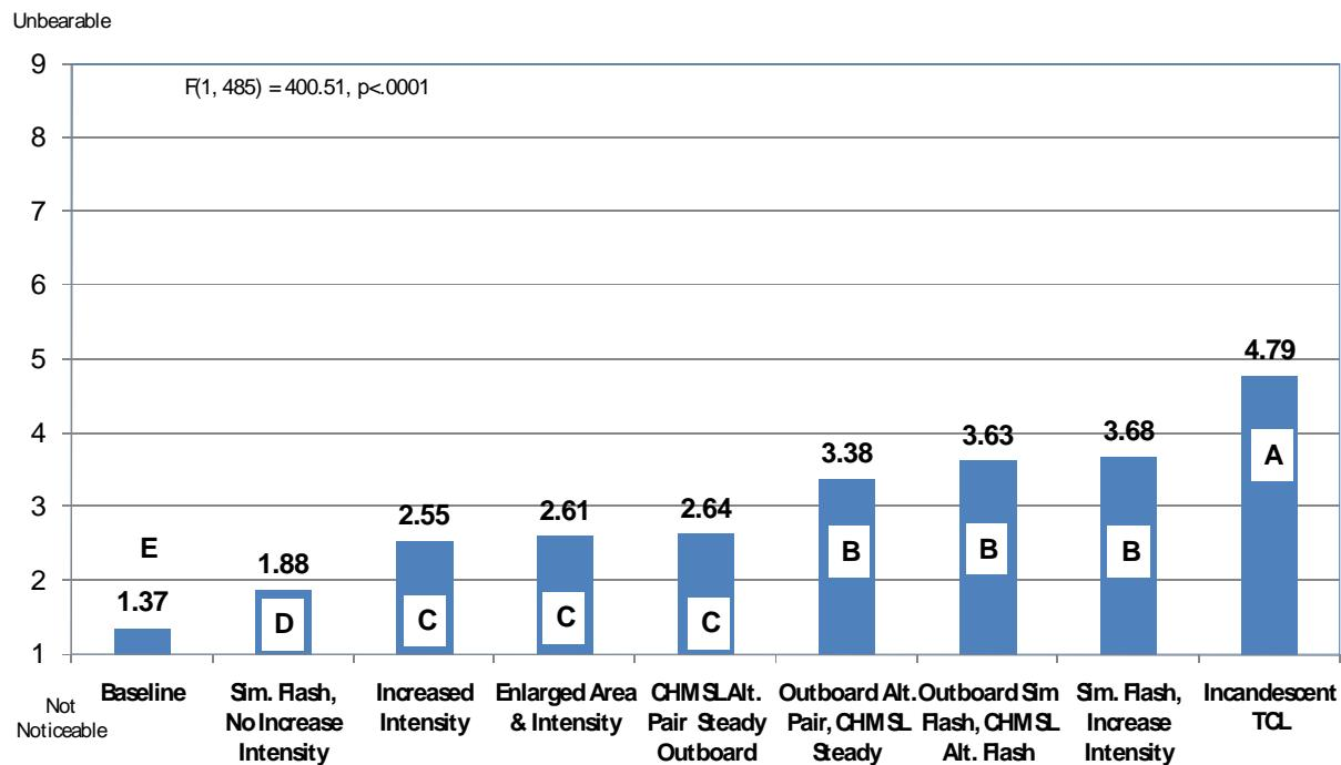
**Figure 34. Main Effect of Lighting Configuration on Discomfort Glare Ratings (in Ascending Order)**
