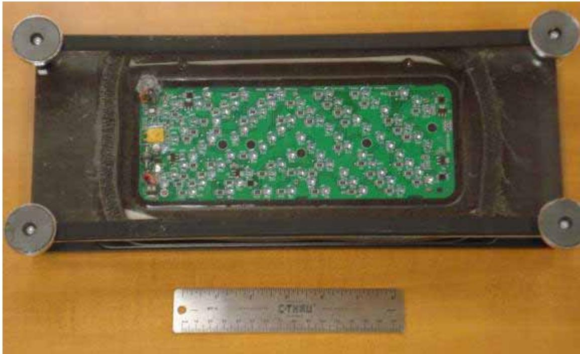
**Figure 4. LED TCL With the Front Bezel and Dispersive Lens Removed, Mounted in Attachment Fixture With Clear Plastic Window**
