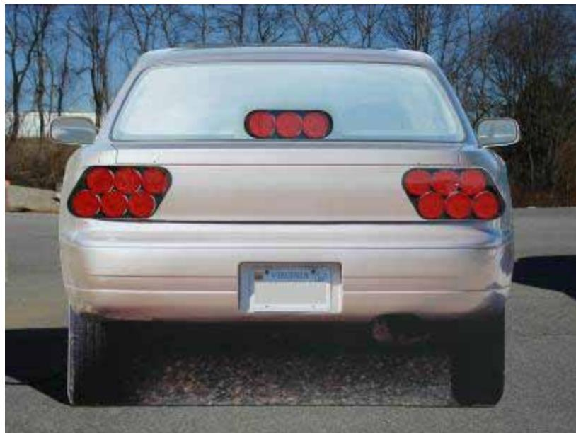
**Figure 6. Test Apparatus Using Three Round Stop Lamps in the CHMSL Position**
