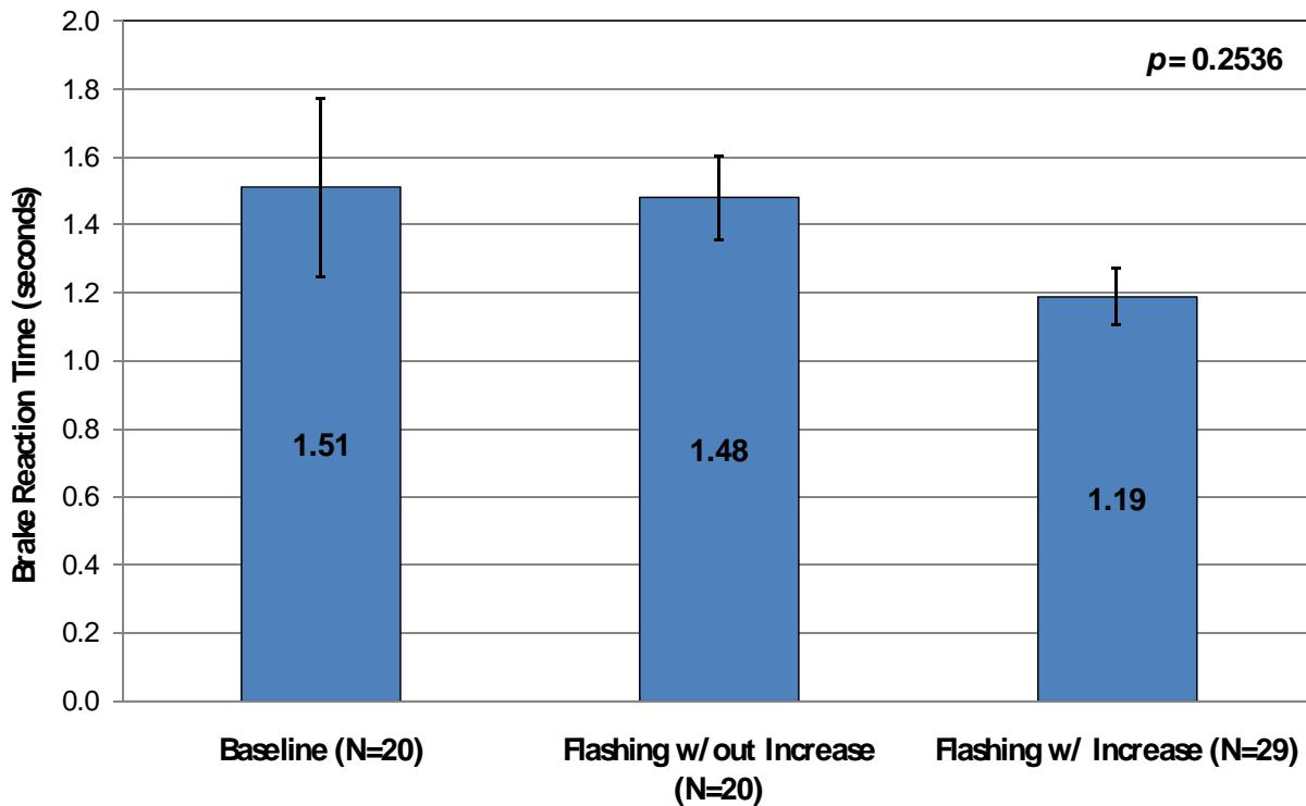
**Figure 49. Mean Brake Response Times Across Lighting Condition (State Route Data Only)**
