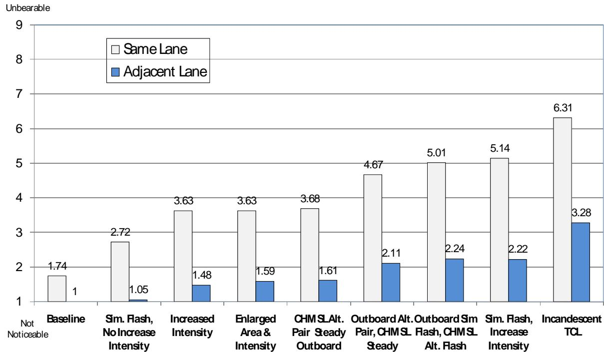
**Figure 33. Effects of Lighting Configuration and Lane Position on Rated Discomfort Glare**
