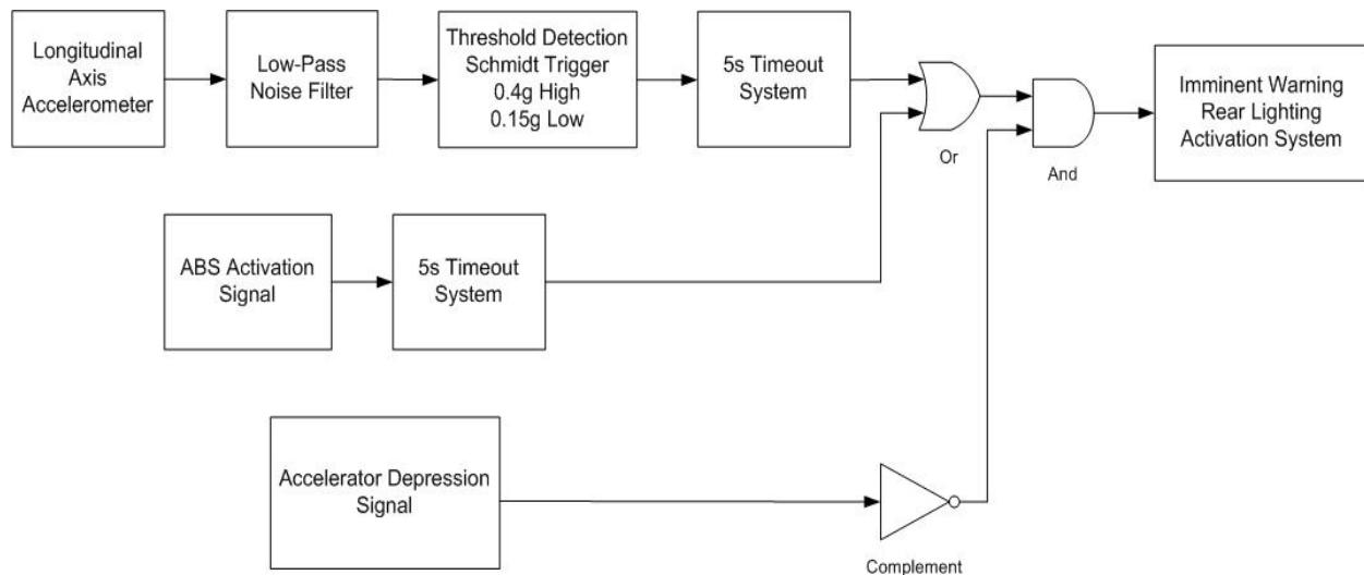
**Figure 60. Block Diagram of the Triggering Logic for the Enhanced Rear Lighting**
