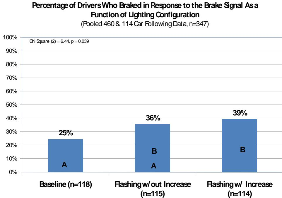
**Figure 46. Percentage of Drivers Observed to Brake in Response to the Brake Signal as a Function of Lighting Condition (Pooled U.S. and State Route Car-Following, n=347)**
