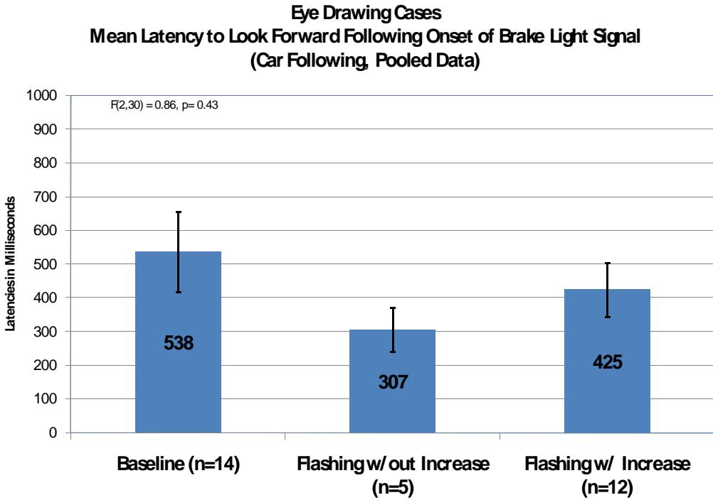
**Figure 43. Mean Response Latencies Across Lighting Condition (Eye-Drawing, Car-Following, and Pooled Data)**
