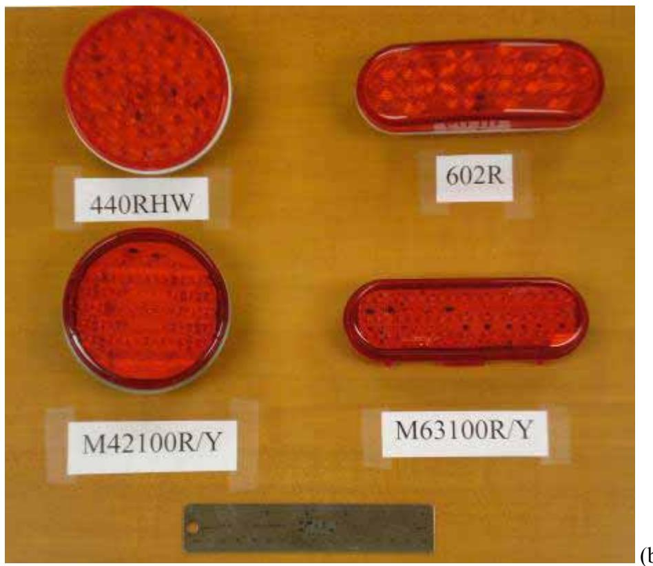
**Figure 3. Rear Lamp Assemblies (a) and Heavy-Vehicle Marker Lamps (b) Tested for Brightness, Beam Width, and Power Consumption**
