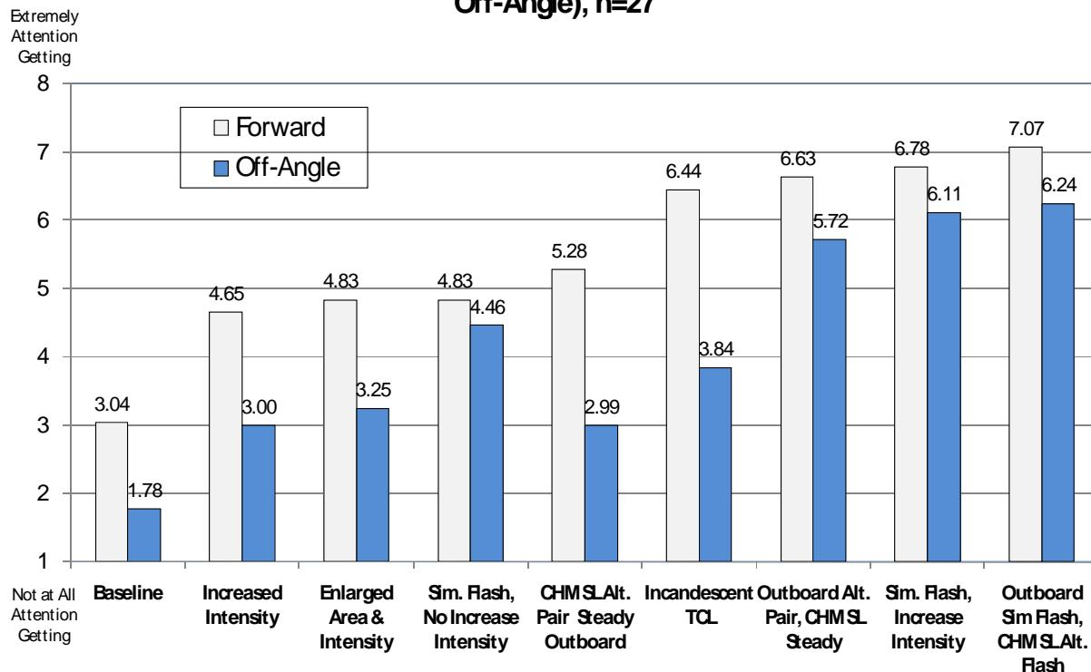
**Figure 31. Attention-Getting Ratings as a Function of Lighting Configuration and Eye Fixation Direction.**
