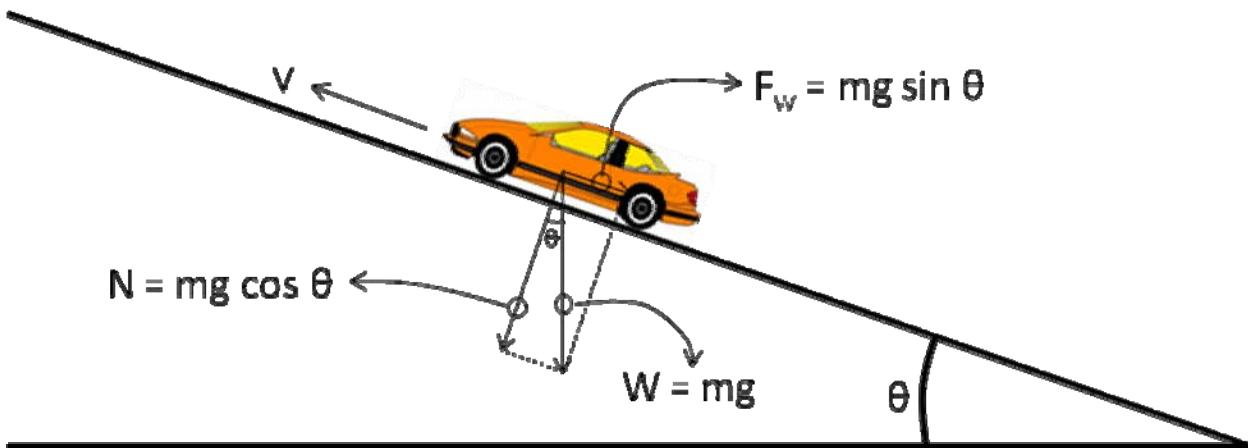
**Figure 57. Forces on a Vehicle created by an Uphill Slope**
