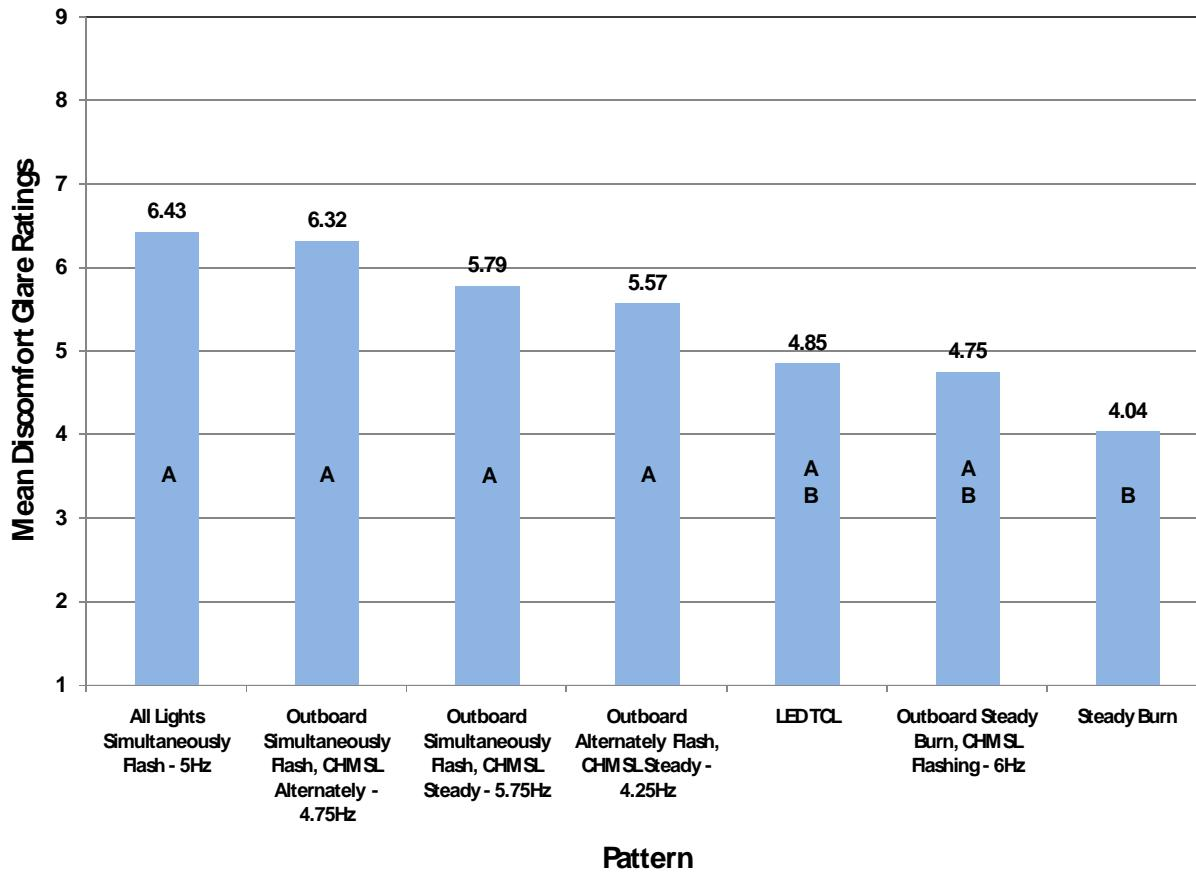
**Figure 16. Results of the Discomfort Glare Ratings at 40 ft (12.2 m) Looking Directly Forward**
