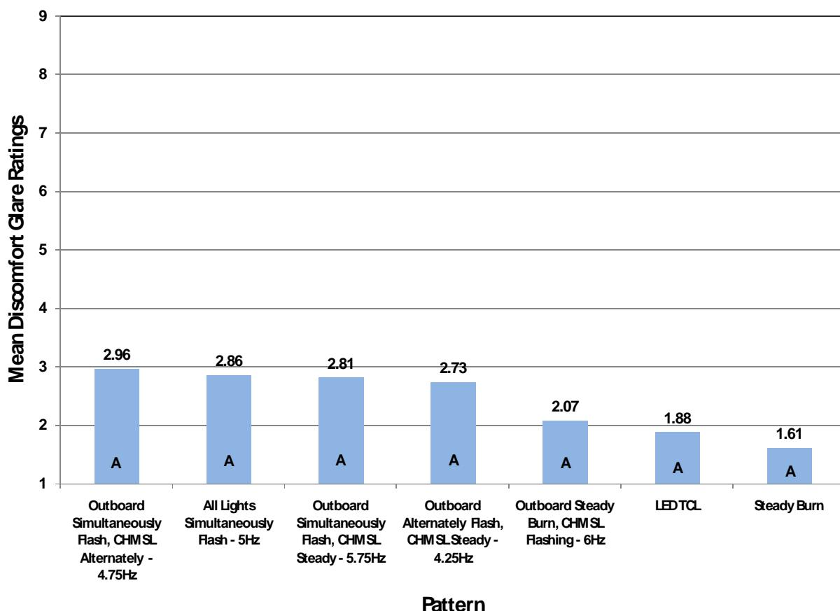
**Figure 17. Results of the Discomfort Glare Ratings at 40 ft (12.2 m), Longitudinal, in the Right Adjacent Lane Looking Straight Forward**
