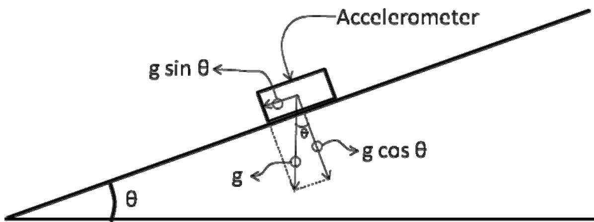
**Figure 58. Effects of a Downhill Slope on a Strapped-Down Accelerometer**
