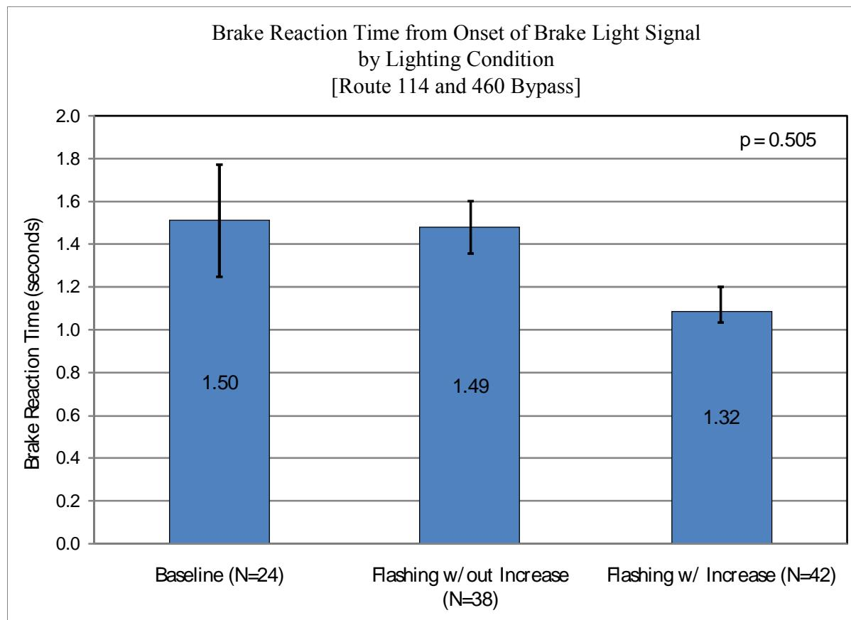
**Figure 48. Mean Brake Response Times Across Lighting Condition (Pooled State and U.S. Route Car-Following Data)**
