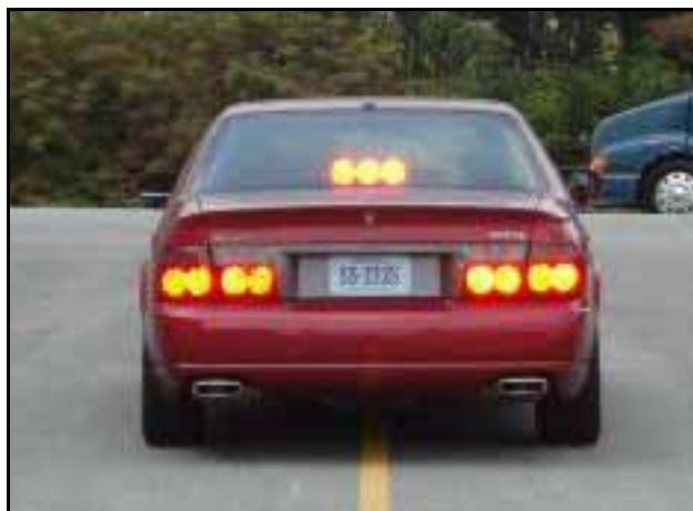
**Figure 38. Research Vehicle With the Rear Lighting Energized at the Emergency Level.
