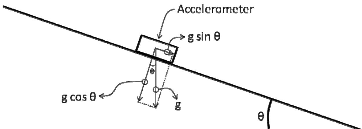
**Figure 59. Effects of an Uphill Slope on a Strapped-Down Accelerometer**
