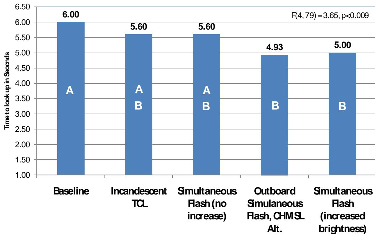
**Figure 24. Mean Look-up Response Times Averaged Across the Three Exposures to the Lighting Display as a Function of Lighting Configuration**
