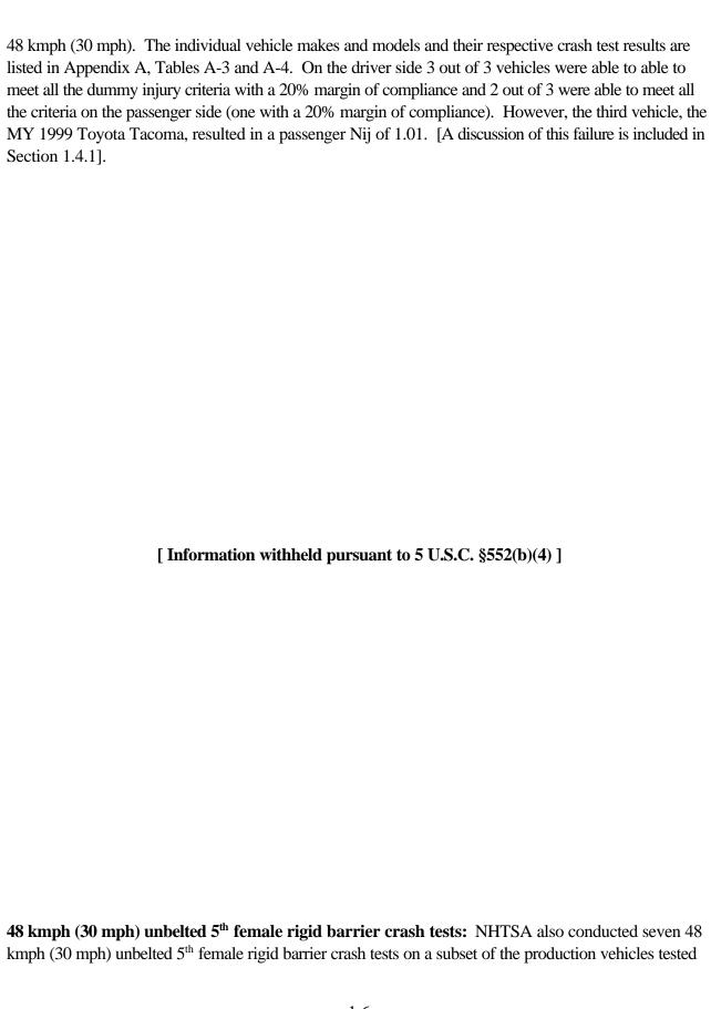
with 50<sup>th</sup> males. The individual vehicle makes and models and their respective crash test results are listed in Appendix A, Tables A-5 and A-6. On the driver side 5 out of 7 vehicles were able to meet all the 5<sup>th</sup> female dummy injury criteria and 4 out of 7 were able to meet all the criteria on the passenger side. Of the 7 vehicles tested, 3 met all of the criteria at both seating positions.
