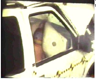
**Figure 7:** Chin-to-instrument panel contact resulting in high passenger dummy Nij.
