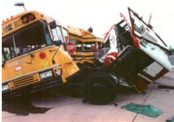
Figure 8. Post Test - Side Impact Crash Test
