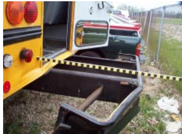
Figure 3. Movement of Bus Body Along the Frame (Rear of Bus Body and Frame)
