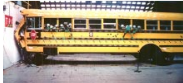
Figure 2. Post-Test Photograph of Frontal Rigid Barrier Crash Test
