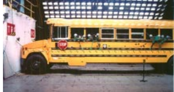
Figure 1. Pre-Test Photograph of Frontal Rigid Barrier Crash Test
