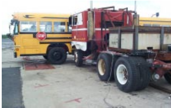
Figure 7. Pre-Test Photograph - Side Impact Crash Test
