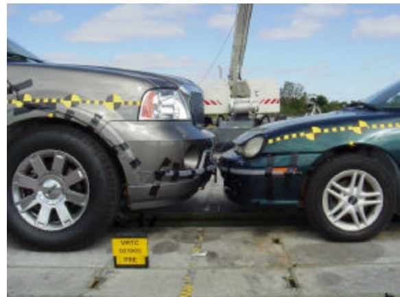
Figure 11. 2003 Navigator pre test alignment
