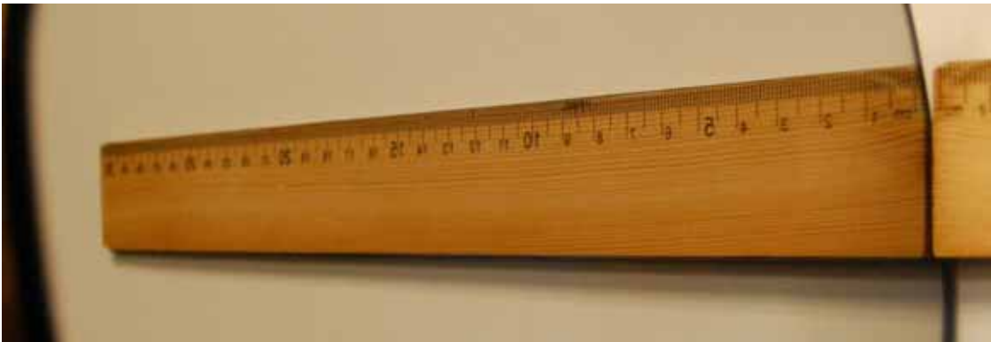
Figure 13. Reference Object Viewed Through a 1400 mm ROC Spherically Convex Mirror
