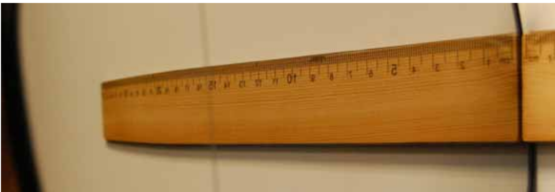
Figure 14. Reference Object Viewed Through a 1400 mm ROC Aspheric Mirror (15 Percent Outboard Aspheric, 85 Percent Inboard Spherically Convex)
