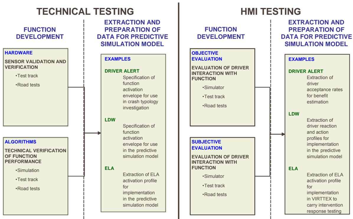
Figure 5.1. Objective testing of ACAT technologies
