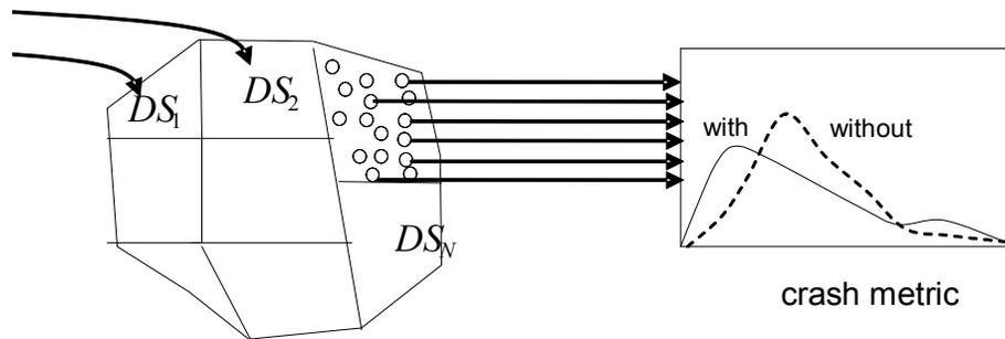
**Figure 10.1. Driving Scenario Resolution for Monte Carlo Simulation With and Without the Specific Safety Technology Being Evaluated.**
