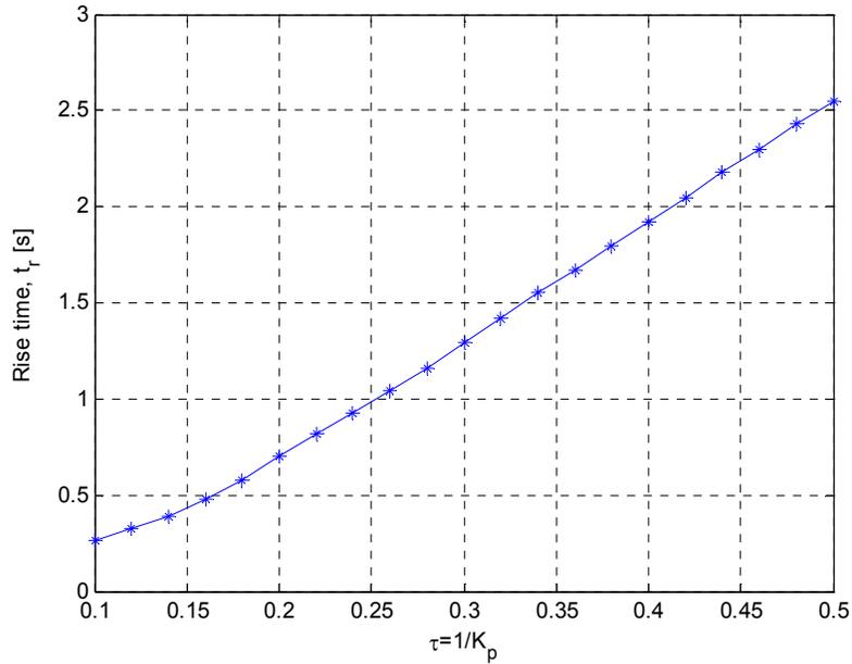
**Figure C.3. Rise Time for Different Control Gains ( $T_s = 0.05$ )**
