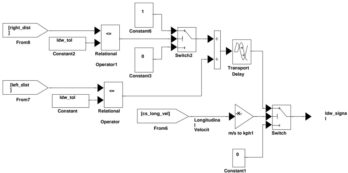
Figure 6.13. LDW System Sub-Model in Simulink
