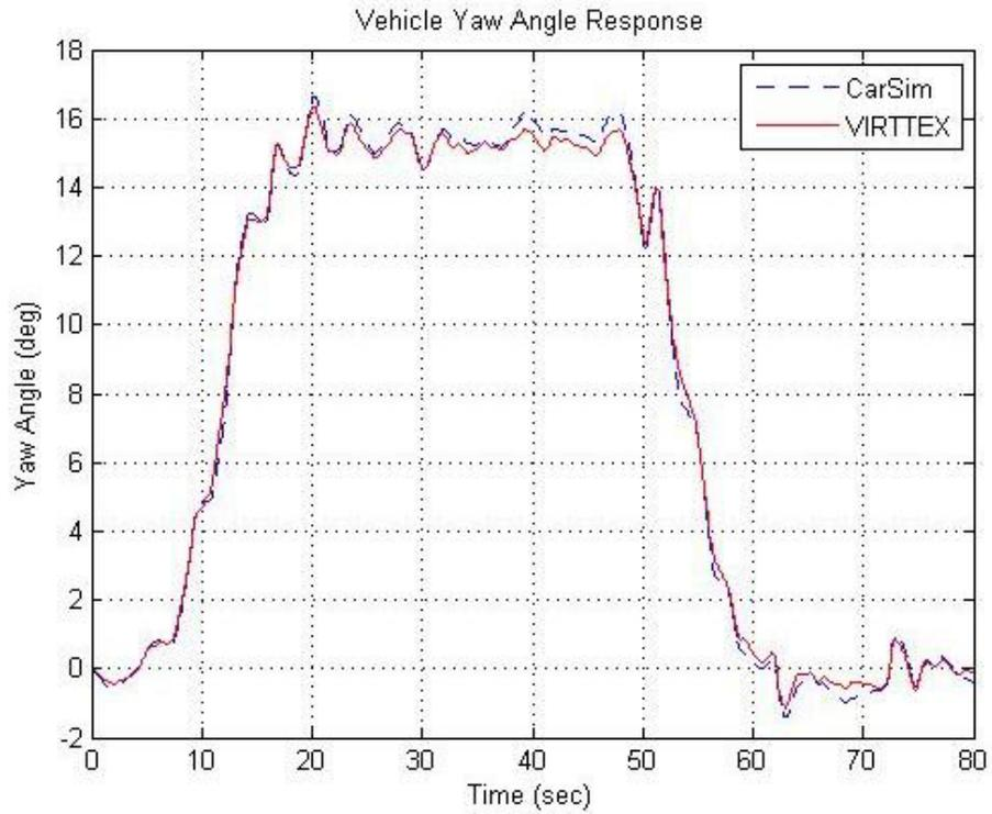
**Figure 6.9. Vehicle Model Yaw Angle Responses to Identical Driver Inputs**
