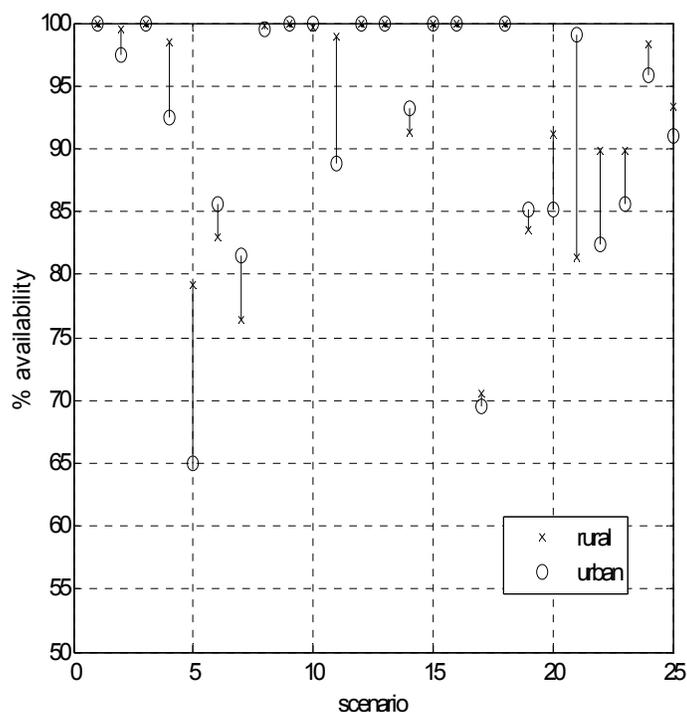
Figure 9.14. Estimated LDW System Availability due to Speed Threshold.
