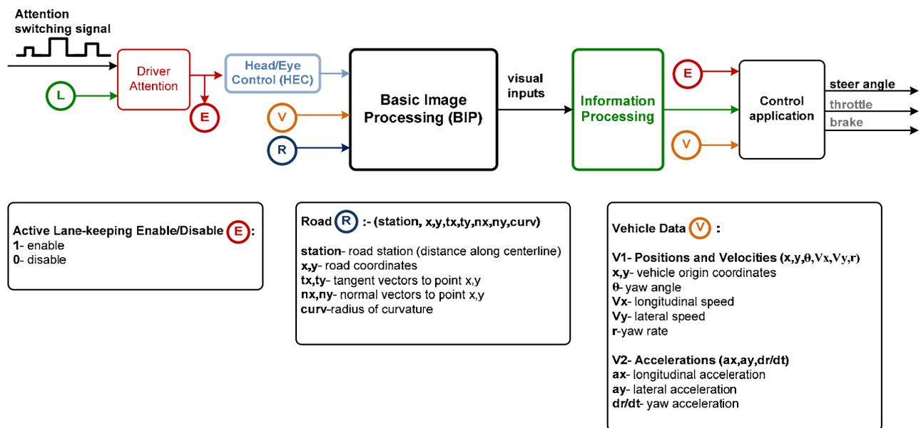
Figure 6.18. Driver Model: Overall Architecture
