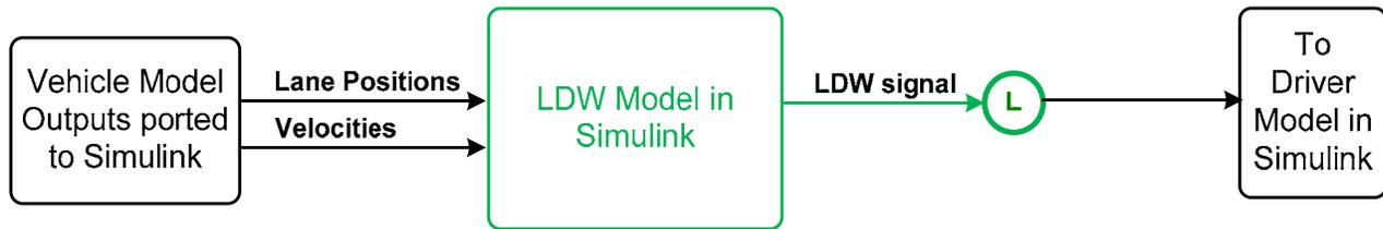
Figure 6.12. Architecture of the LDW Model
