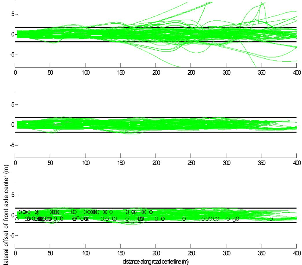
**Figure 8.4. Effect of LDW on Lane-keeping. Trajectories shown for Scenario 1, Rural, left travel lane(upper plot: no LDW, center plot with LDW, lower plot also shows the location where the LDW alert is issued)**
