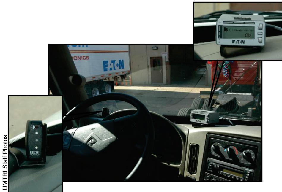
Figure 1. Driver-vehicle interface of the integrated safety system
